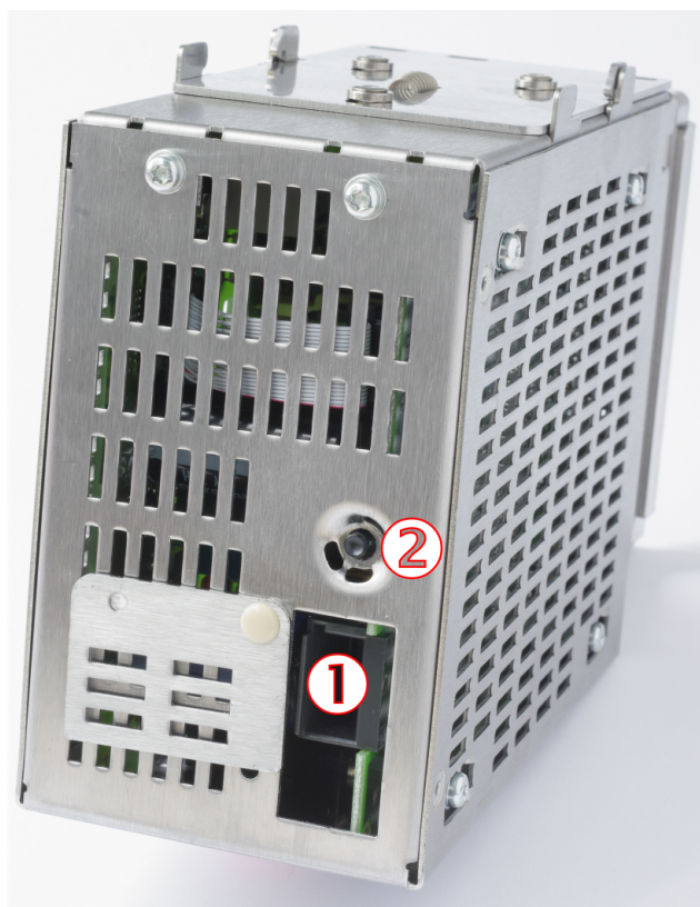
Figure 5-9 Position of the C-PLUG and SELECT/SET button
