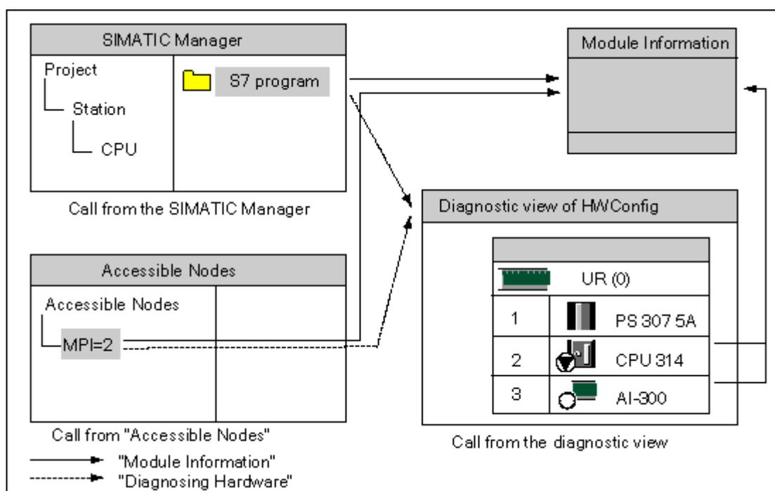
In order to display the status of a **module with its own node address**, you require an online connection to the programmable controller. You establish this connection via the online view of a project or via the "Accessible Nodes" window.
