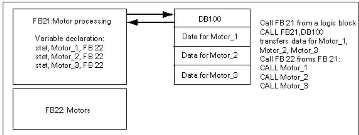
In this example, FB22 does not need its own instance data block, since its instance data are saved in the instance data block of the calling FB.
