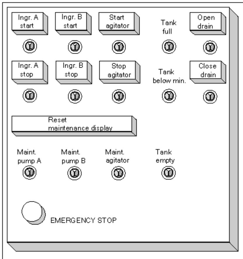
The console also includes display lamps for the devices that require maintenance after a certain number of starts and the emergency off switch with which the process can be stopped immediately. The console also has a reset button for the maintenance display of the three motors. Using this, you can turn off the maintenance display lamps for the motors due for maintenance and reset the corresponding counters to 0.
