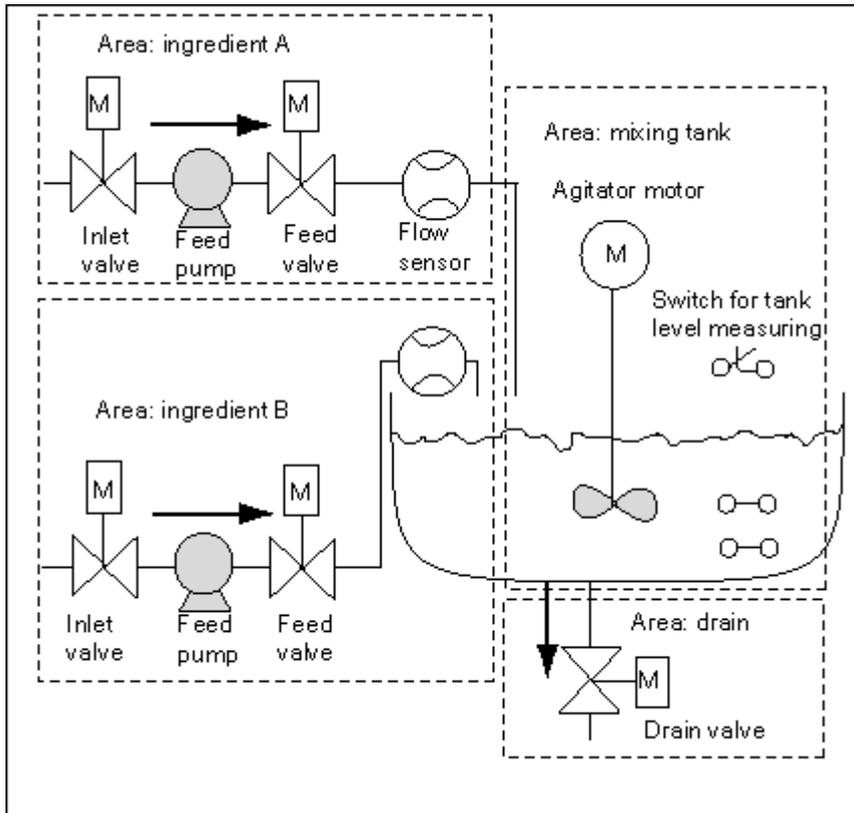
As each group is divided into smaller tasks, the tasks required for controlling that part of the process become less complicated.
