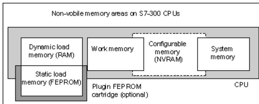
To do this set the CPU so that the following data are saved in the nonvolatile RAM:
