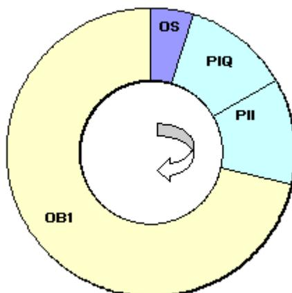
One of the internal tasks of the operating system (OS) is to write the process image output table (PIQ) to the outputs for the modules and to read in the status of inputs into the process image input table (PII). Once this step is complete, the user program is executed with all blocks that are called in it. Writing the process image output table to the outputs for the modules and reading in the process image input table is all independently controlled by the operating system.
