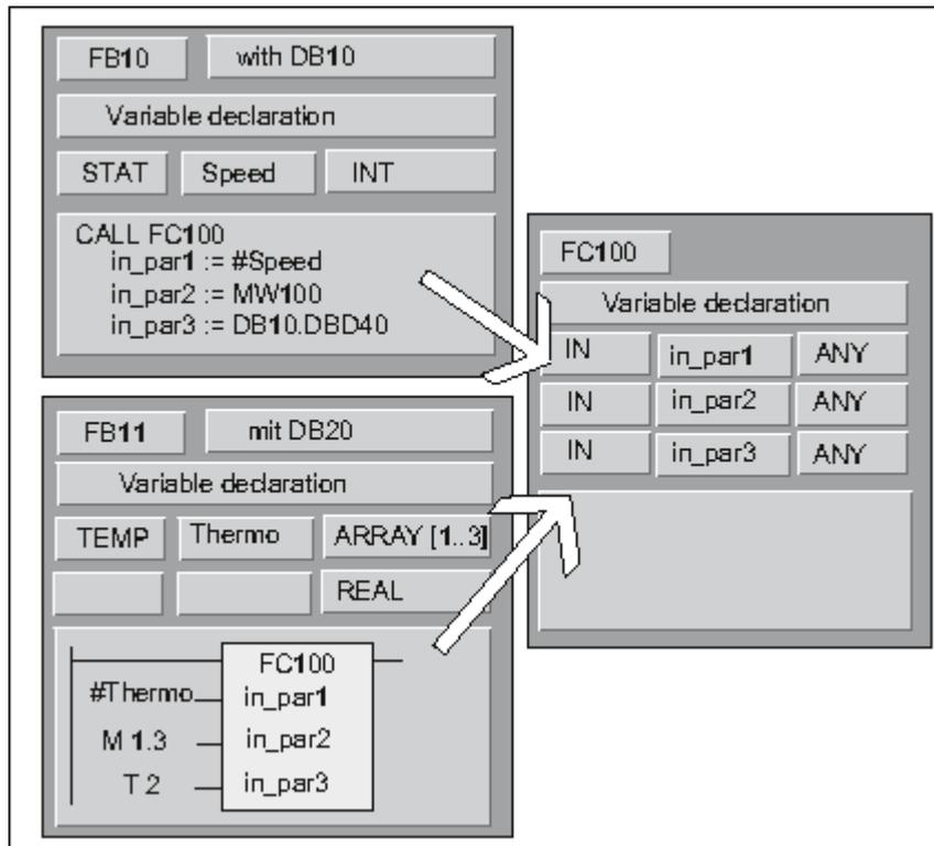
In this example, FC100 has three parameters (*in\_par1*, *in\_par2*, and *in\_par3*) declared as the ANY data type.
