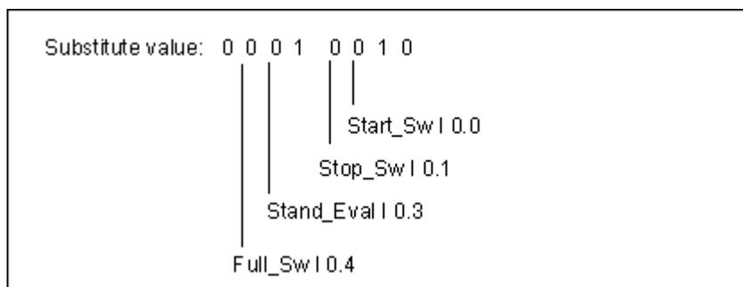
If an input module fails, the processing of the statement L PIB0 produces a synchronous error and starts OB122. As standard, the load instruction reads in the value 0. With SFC44, however, you can define any substitute value suitable for the process. The SFC replaces the accumulator content with the specified substitute value.
