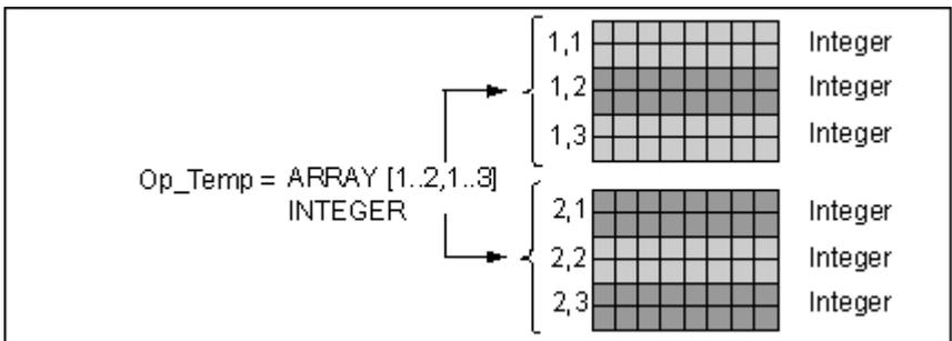
You access the data in a multi-dimensional array using the index. In this example, the first integer is `Op_temp[1,1]`, the third is `Op_temp[1,3]`, the fourth is `Op_temp[2,1]`, and the sixth is `Op_temp[2,3]`.
