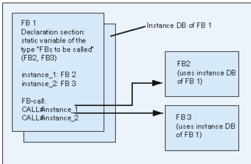
Only requirement: You must "tell" the calling function block which instances you are calling and what (FB) type these instances are. These details must be entered in the declaration window of the calling function block. The function block used must have at least one variable or parameter from the data area (VAR\_TEMP cannot be used).
