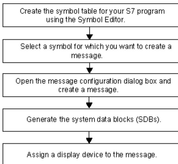
During processing, the signals for which you have configured messages are checked asynchronously to your program. The checks take place at the configured time intervals. The messages are displayed on the assigned display devices.
