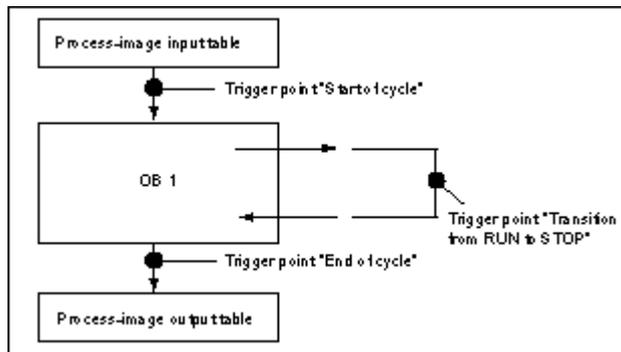
To display the modified value in the "Status Value" column, you should set the trigger point for monitoring to "Start of cycle" and the trigger point for modifying to "End of cycle".
