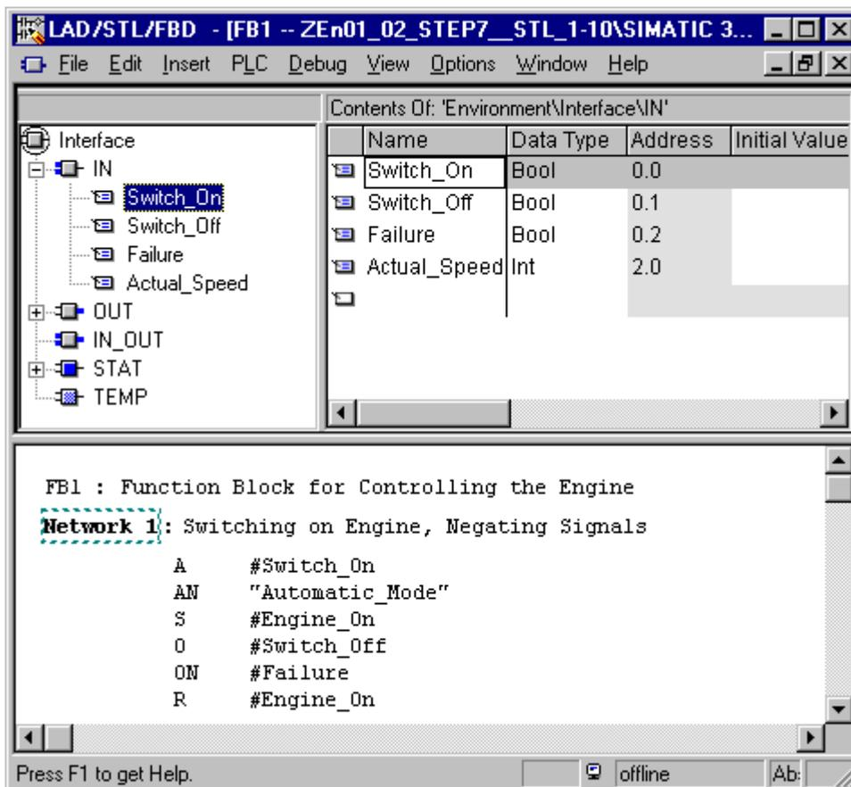
In the variable detail view, you specify the local variables and the formal parameters for the block as well as the system attributes for parameters. This has the following effects:
