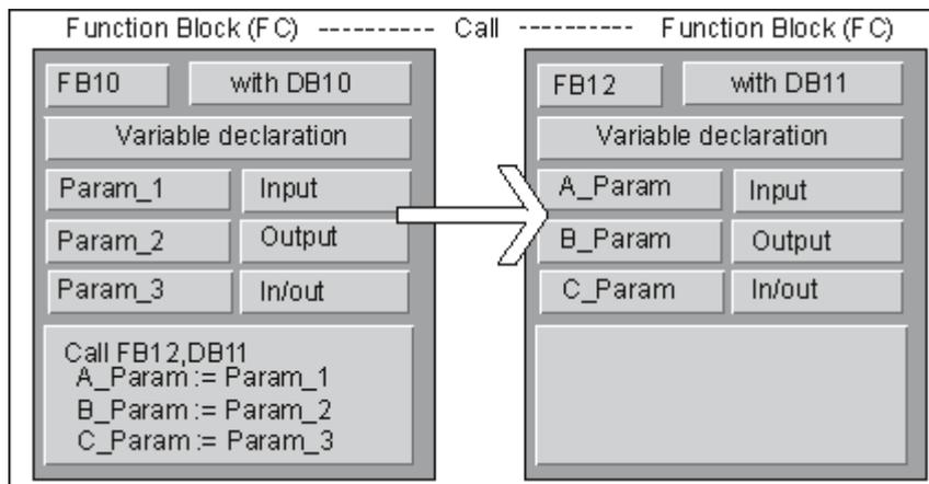
STEP 7 restricts the assignment of the formal parameters of an FB to the formal parameters of another FB. You cannot, for example, assign input and output parameters with complex data types as the actual parameters for the input and output parameters of a called FB. You can, however, assign input parameters of the parameter types TIMER, COUNTER, or BLOCK to the input parameters of the called FB.
