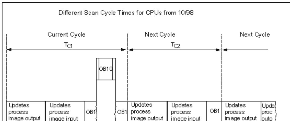
In the current cycle, OB1 is interrupted by a time-of-day interrupt.
