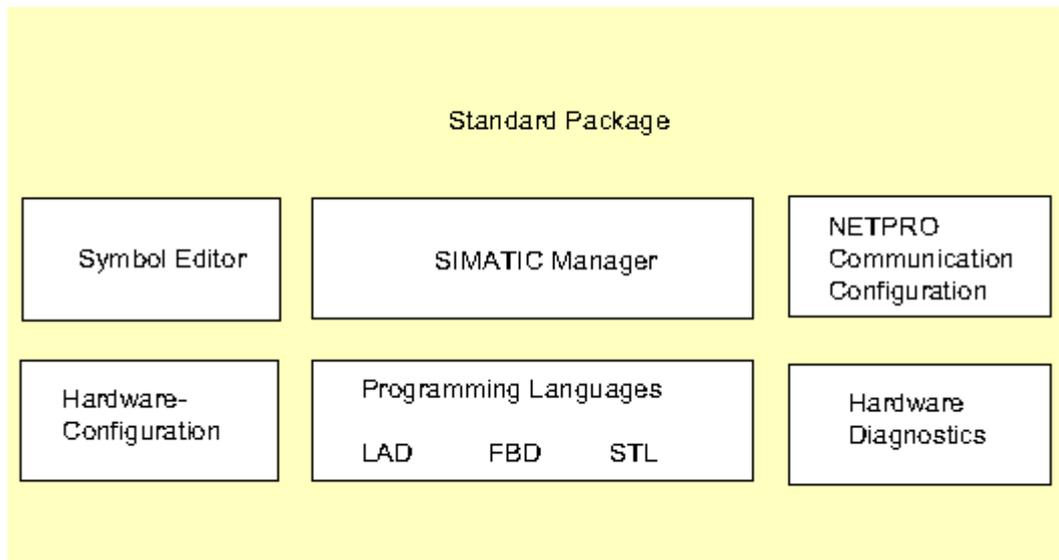
You do not need to open the tools separately; they are started automatically when you select the corresponding function or open an object.
