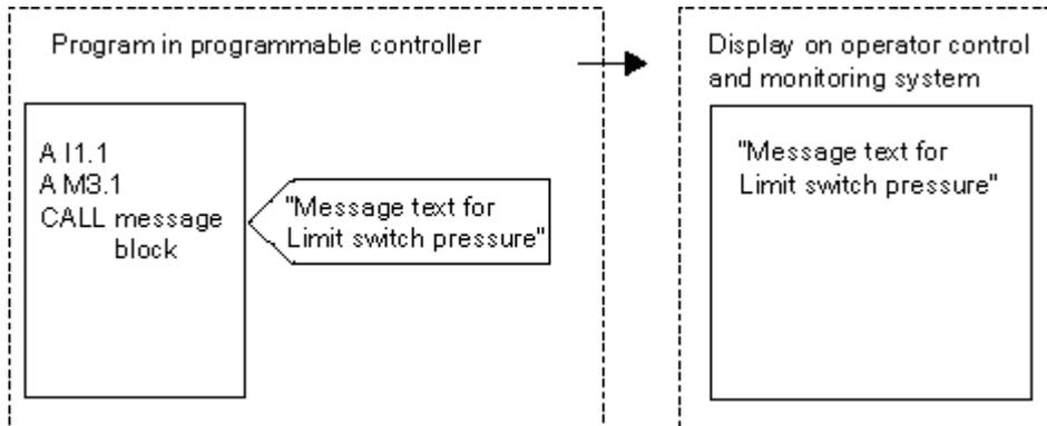
There is no cyclic query of the programmable controller. When the programmable controller signals a change, the corresponding message number is passed to the operator interface system and the corresponding message text is displayed. The message receives the time stamp from the programmable controller and can therefore be traced more exactly than with bit messaging.
