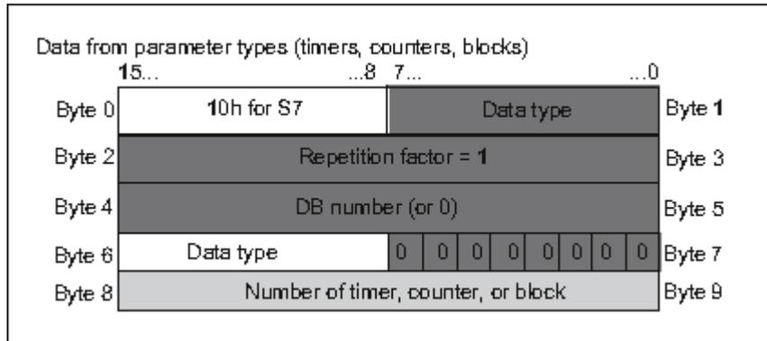
The following table shows the coding of the data types for the parameter type ANY for parameter types.
