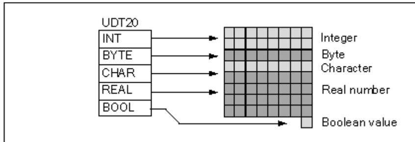
Instead of entering all the data types singly or as a structure, you only need to specify "UDT20" as the data type and STEP 7 automatically assigns the corresponding memory space.
