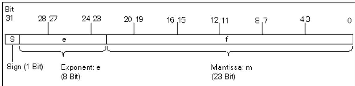
The following table shows the values of the individual bits in floating-point format.
