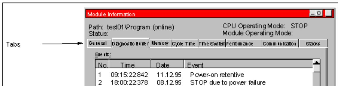
The names of the tab cards are shown on tabs along the top edge of the dialog box. To bring a particular tab card to the foreground, you simply click on its tab.
