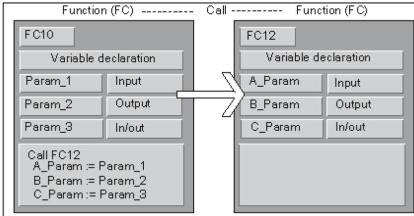
STEP 7 restricts the assignment of formal parameters of an FC as actual parameters for the formal parameters of a different FC. You cannot, for example, assign parameters with complex data types or a parameter type as the actual parameter.
