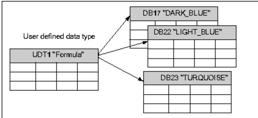
The structure of the data block is determined by the UDT assigned to it.
