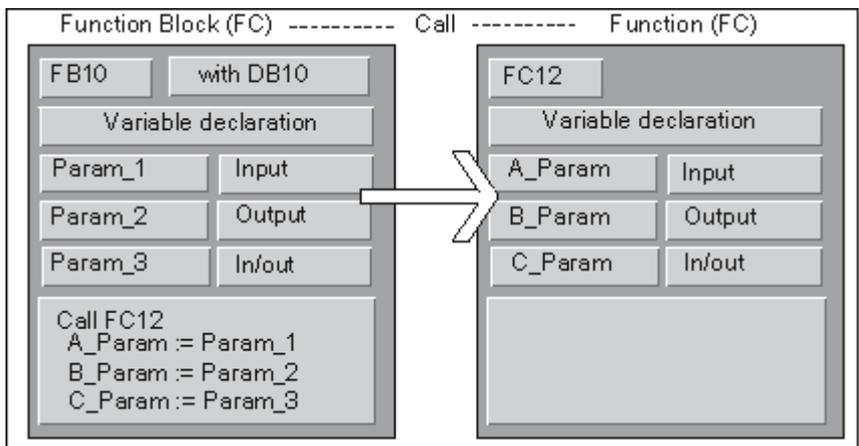
STEP 7 restricts the assignment of the formal parameters of an FB to the formal parameters of an FC. You cannot, for example, assign parameters of the parameter type as actual parameters. The following table shows the permitted data types (●) when an FB calls an FC.
