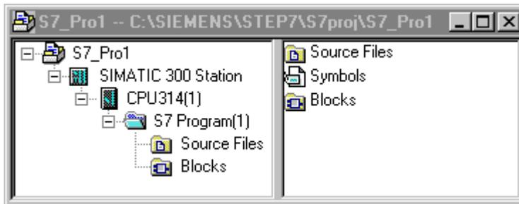
You can display the project structure for the data available on the programming device in the component view "offline" and for the data available on the programmable control system in the component view "online" in project windows.
