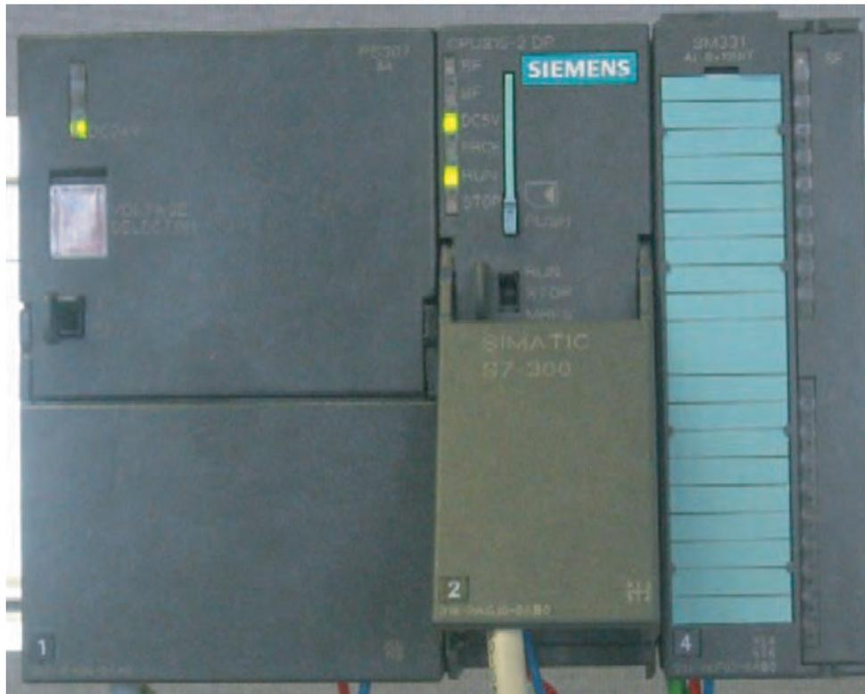
Figure 6-13 CPU in error free state
