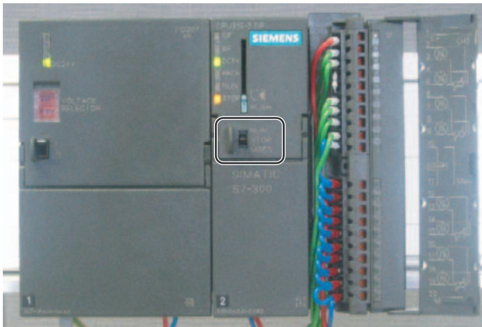
Figure 5-5 câblage correct, CPU en STOP
