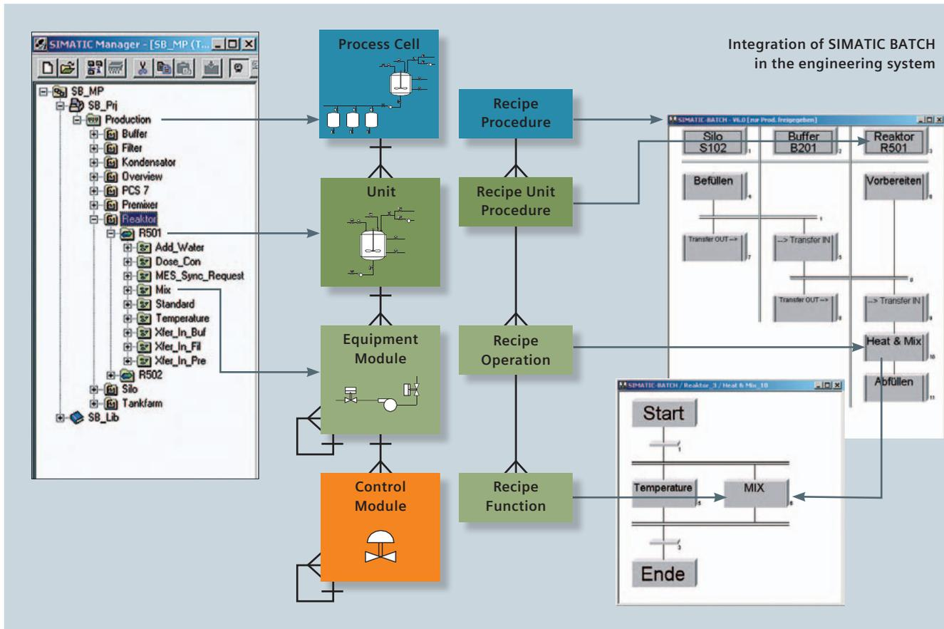
The creation of unit or device neutral recipes, that can be used on several production devices of the same type, provides you with two simultaneous advantages: the engineering cost is significantly reduced and validation is greatly simplified. The assignment of the current production equipment is implemented at the batch level. For you as the user, this means the highest level of flexibility and simple adaptation to individual plant situations:
