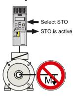
The inverter with active STO function prevents machine components from inadvertently starting.
