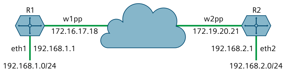
Figure 12.6 Example – GRE Tunnel Configuration
