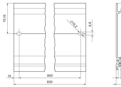
Figure A-5 Mounting rail 830 mm
