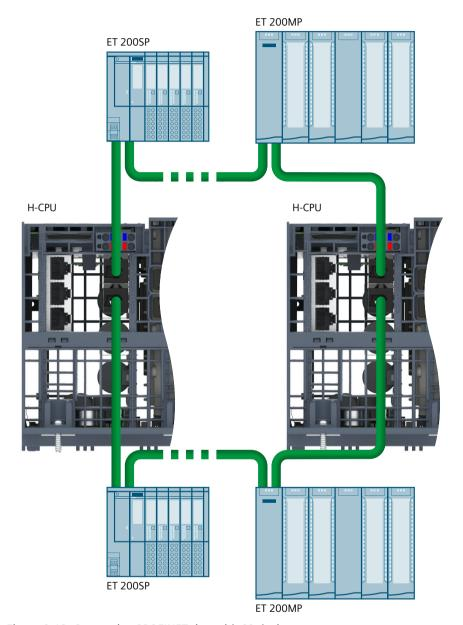
Figure 8-13 Connecting PROFINET ring with S2 devices
