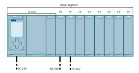
Figure 6-70 Configuration example of H-CPU with redundant system power supplies and 6 CPs
