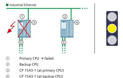
§ PROFINET cable (redundancy connections, PROFINET ring) Figure 6-35 S7-1500R failure of the primary CPU with CP 1543-1
