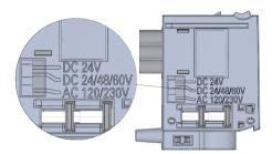
Figure 14-4 Labeling on the power connector
