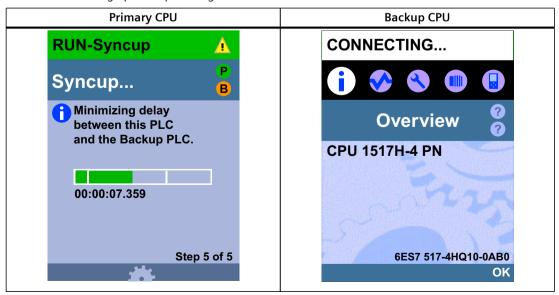
Once the backup CPU has caught up, both CPUs switch to the RUN-Redundant mode. The backup CPU establishes connections to the IO devices (only with system redundancy S2 and R1) and the communication links are available again. Both CPUs process the user program synchronously.
