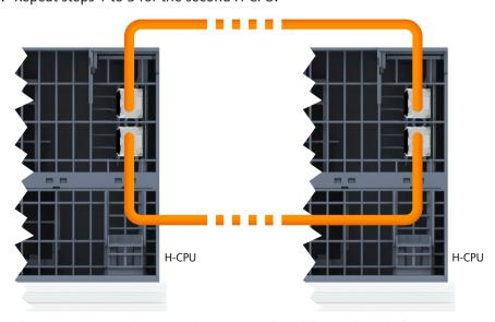
Figure 8-12 Connecting redundancy connections (fiber-optic cables) to S7-1500H
