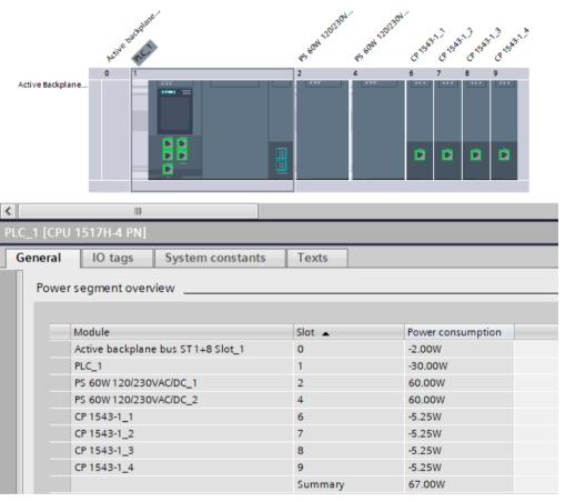
Figure 6-71 Power segment overview with redundant system power supplies
