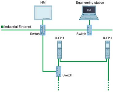
Figure 6-66 Configuration example CPU 1513R-1 PN: Connecting the HMI device via a switch CPU 1513R-1 PN has a PROFINET IO interface with 2 ports (X1 P1R R and X1 P2R).
