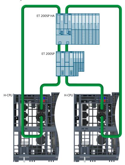
Figure 8-14 Connecting PROFINET rings with R1 devices
