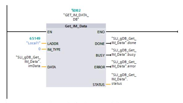
Figure 12-15 Example: Read out I&MO data from the S7-1500R redundant system
