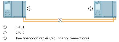
Figure 6-30 S7-1500H configuration with additional devices
