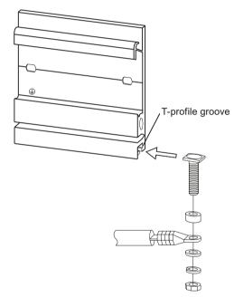
Figure 7-3 Attaching the protective conductor (protective earth)
