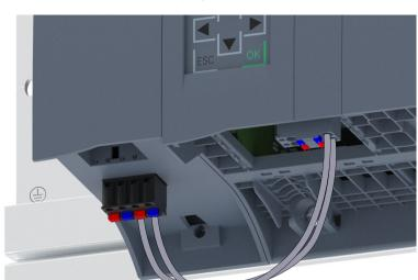
3. Connect the load current supply to the CPU.
