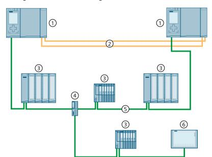
The figure below shows a configuration of the S7-1500H with S2 devices in a line topology.
