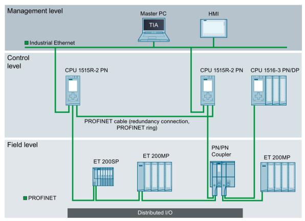
Figure 5-11 Possible configuration at the management, control and field level using the example of S7-1500R
