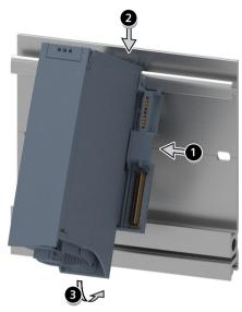
Figure 7-9 Installing a system power supply
