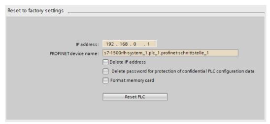
Figure 4-1 Resetting the CPU to factory settings
