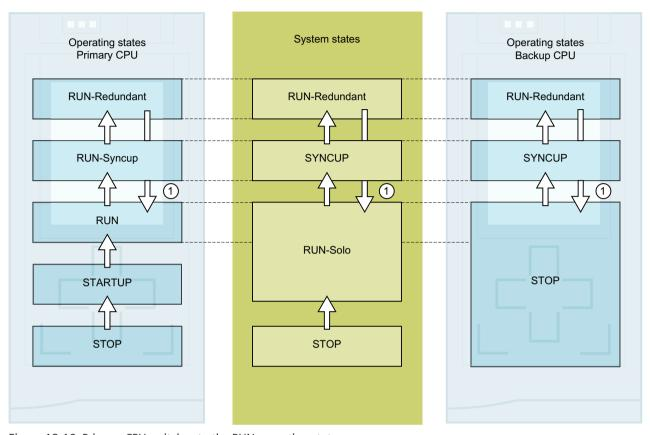
Figure 12-10 Primary CPU switches to the RUN operating state
