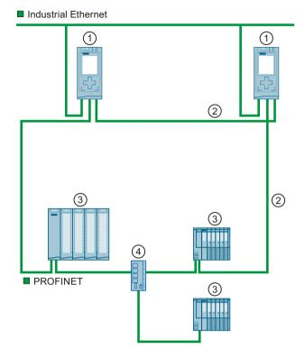
The following figure shows a configuration of the S7-1500R in the PROFINET ring.
