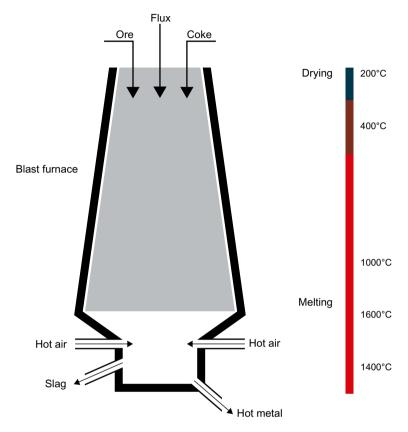
Figure 5-3 Example: Blast furnace
