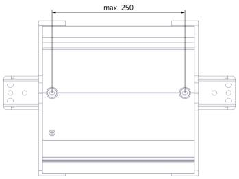
Figure 7-6 Distance between two DIN rail adapters
