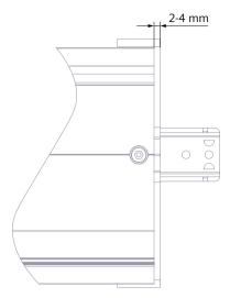
Figure 7-7 DIN rail adapter protrusion
