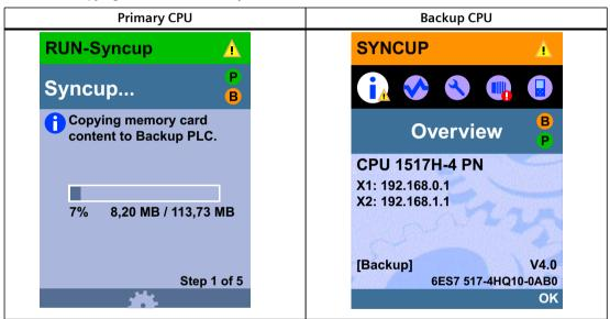
The backup CPU copies the transferred load memory contents to its work memory.
