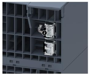
Figure 8-11 Inserting and locking synchronization modules
