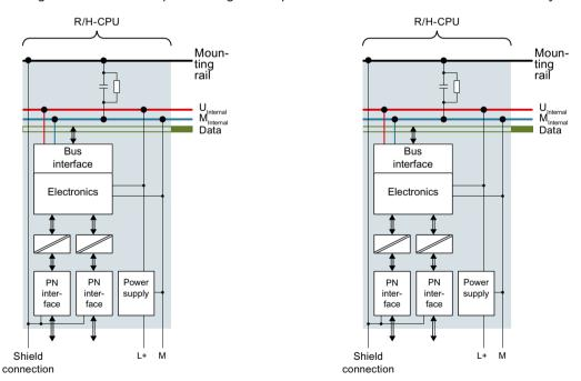
Figure 8-2 Potentials in S7-1500R/H using the example of CPU 1515R-2 PN
