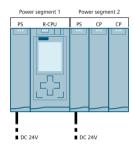
Figure 6-67 Configuration example R-CPU with 2 system power supplies
