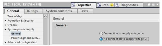
Figure 9-15 Connecting PS 60W 24/48/60VDC HF
