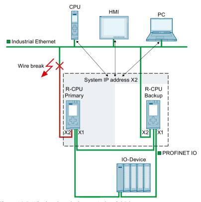
Figure 10-5 Wire break to devices on Industrial Ethernet
