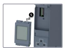
14.2 Replacing the display/front cover
