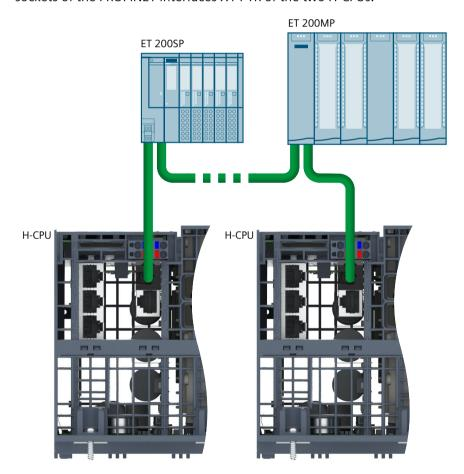
Figure 8-15 Connect line topology with S2 devices to S7-1500H
