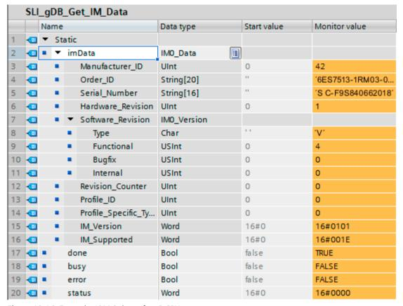
Figure 12-16 Example: I&M 0 data of an R CPU
