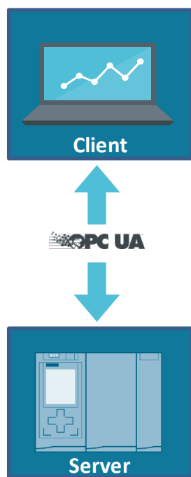
Figure 2-1: OPC UA client and server architecture
