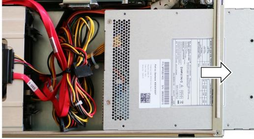
7. Remove the cable ties securing the power cables in the enclosure.
