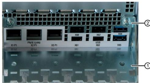
3. Insert detachable cable ties into corresponding holes of the strain relief and secure the cable with the cable ties.
