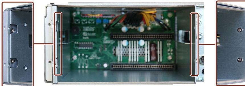
5. Loosen the screws marked in the following picture at the enclosure bottom.
