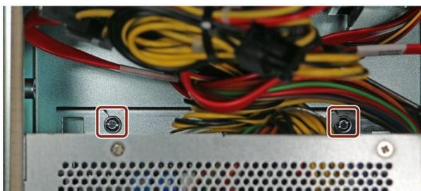
6. Pull the enclosure a bit towards the front so that the cables can be accessed.
