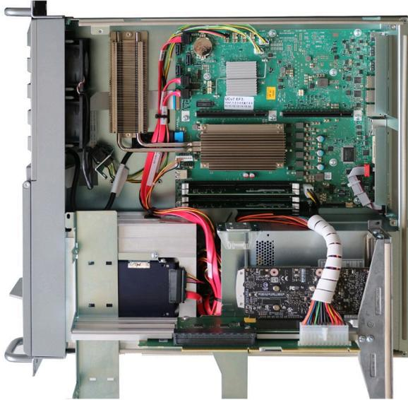
6. Unlock the power supply plug and disconnect it.
