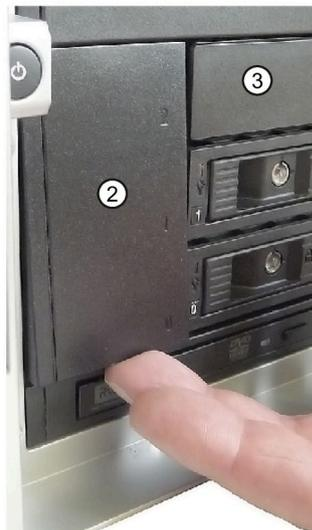
6. On the front of the drive cage, remove the cover of the mounting locations ③, which may be located to the right of the cover ②.
