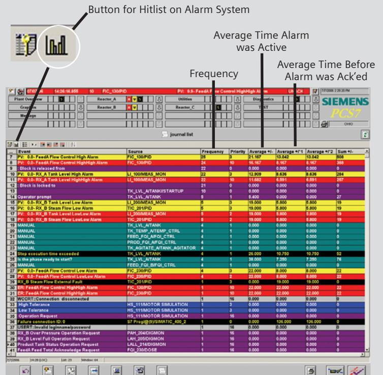
Figure 9 Alarm Frequency Analysis Helps Identify "Nuisance" Alarms
