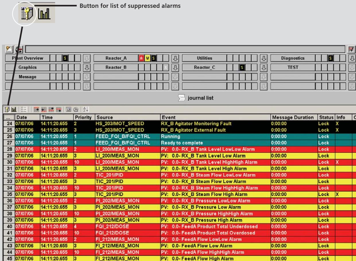
Figure 5 List of Suppressed Alarms (Locked)
