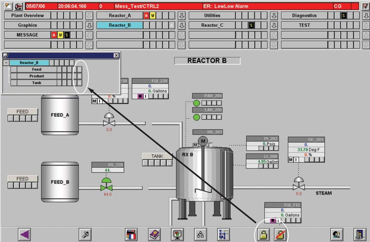
Figure 4 Operator Interface Showing Alarms Suppressed in a Process Area
