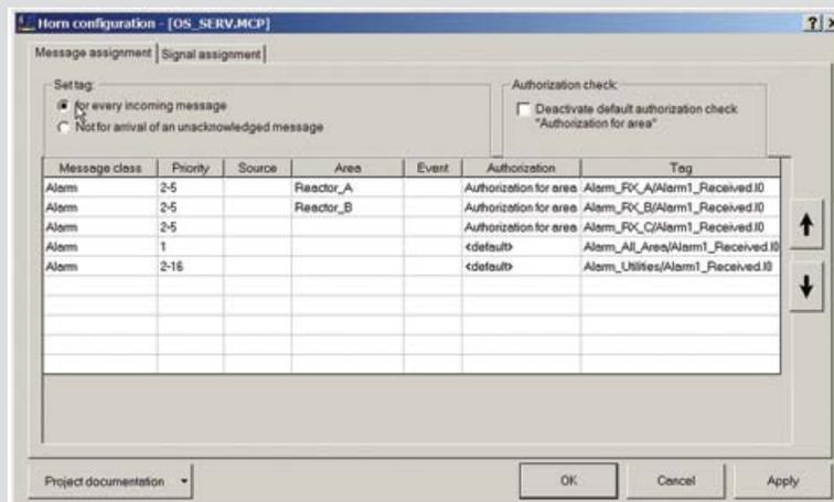
Figure 2 Alarm Horn Configuration Tool
