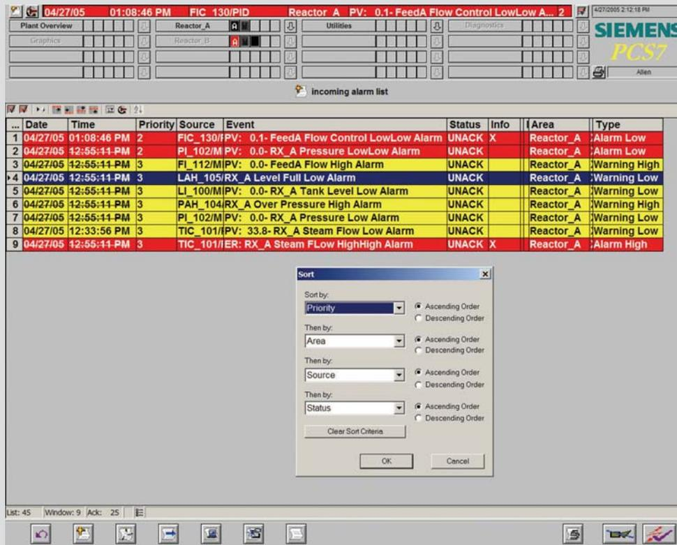
Figure 1 Filtering and Sorting of Alarms in the Incoming Alarm List
