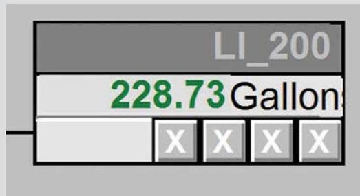
Figure 3 Standard HMI Symbol with Alarms Suppressed
