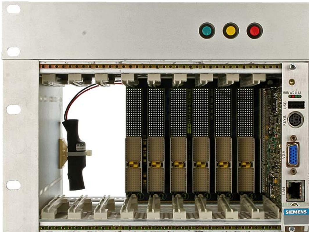
4. Attach the connectors for the flat ribbon cables used for communication between the basic module and the I/O modules to the basic module.
