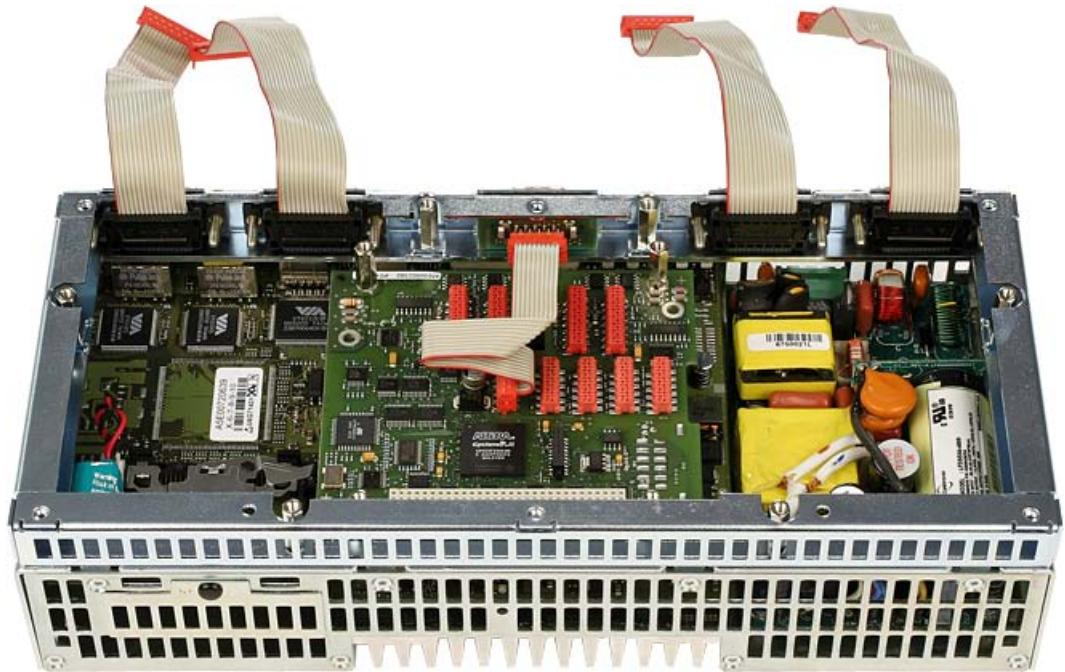
*5.3 Installation example: Basic module, encoder rack and four I/O modules*
