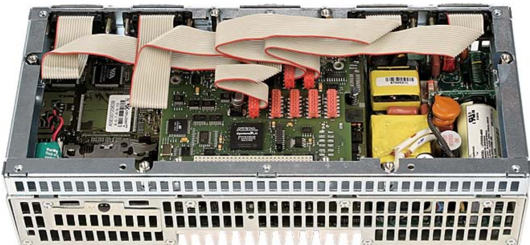
*5.3 Installation example: Basic module, encoder rack and four I/O modules*
