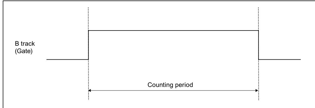
Figure 7-3 Level-controlled gate generation
