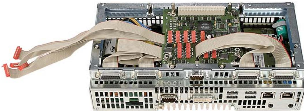
13. Install the first I/O expansion rack. Tighten the six 21 mm M3 stud bolts (width across flats 5).
