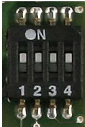
Figure 5-1 Slot selection switch
