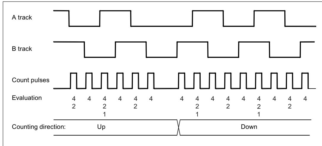
Figure 7-1 Shaft encoder edge evaluation without hysteresis function
