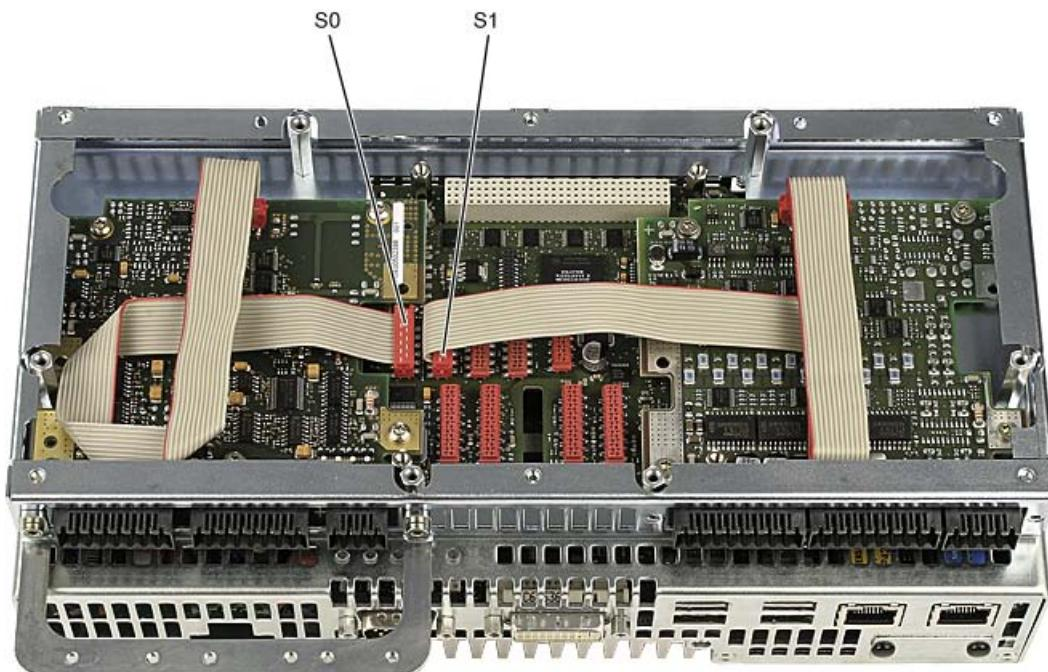
8. Check that all ribbon cable connectors are correctly seated
