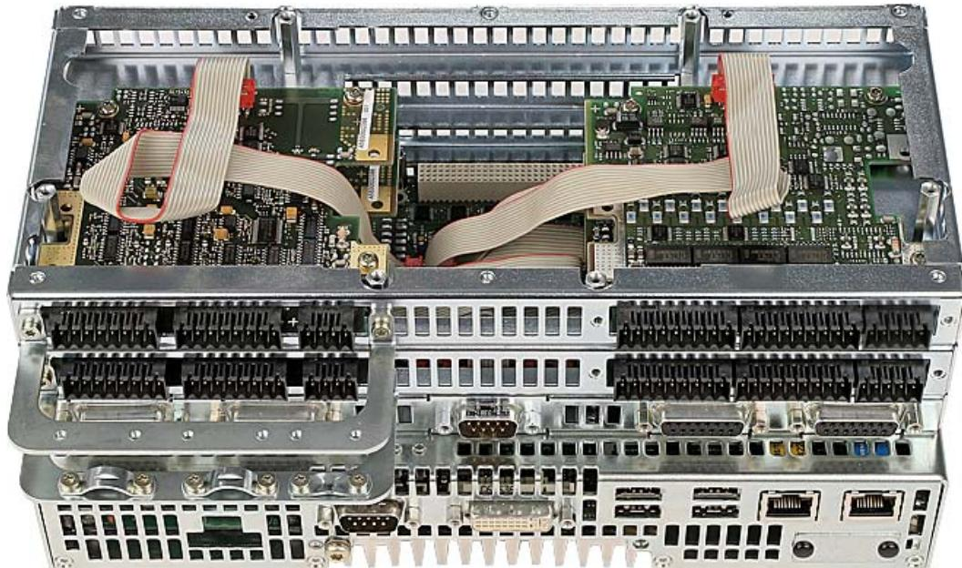
13. Check that all ribbon cable connectors are correctly seated
