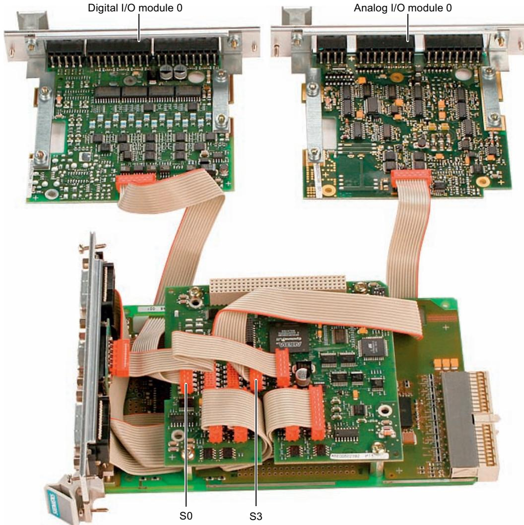
*6.2 Installation example: Basic module and two I/O modules*
