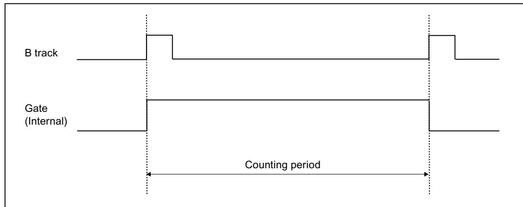
Figure 7-4 Edge-controlled gate generation
