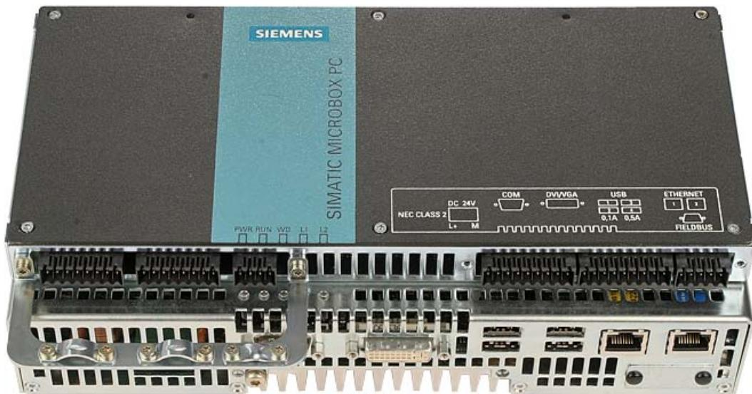
14. Connect the external 24 V power supply for the digital I/O module 0. The digital I/O module 0 will not work without this power supply.
