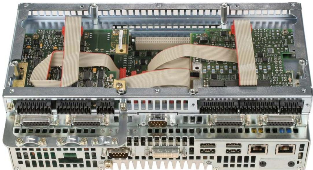
**5.3 Installation example: Basic module, encoder rack and four I/O modules**
