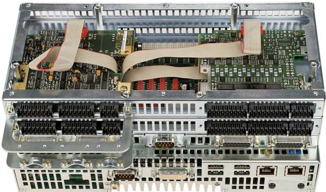
17. Install the third I/O expansion rack. Tighten the six 21 mm M3 stud bolts (width across flats 5).
