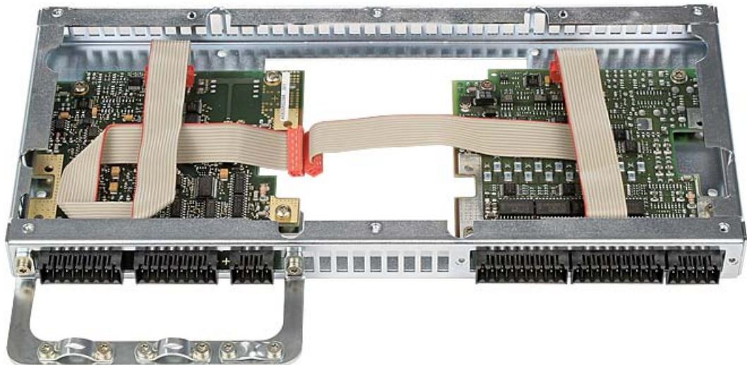
10. Install the set-up I/O expansion rack. Tighten the six 21 mm M3 threaded bolts (width across flats 5).
