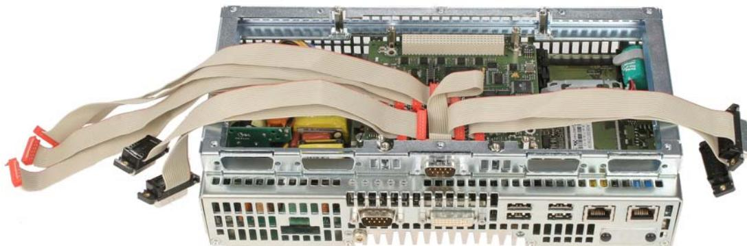
7. Fasten the 9-pin sub D connector for the encoder power supply interface to the encoder expansion rack as shown in the figure above.
