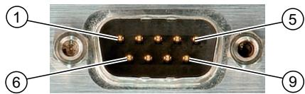
Table 11-18 Encoder inputs/9-pin sub D connector
