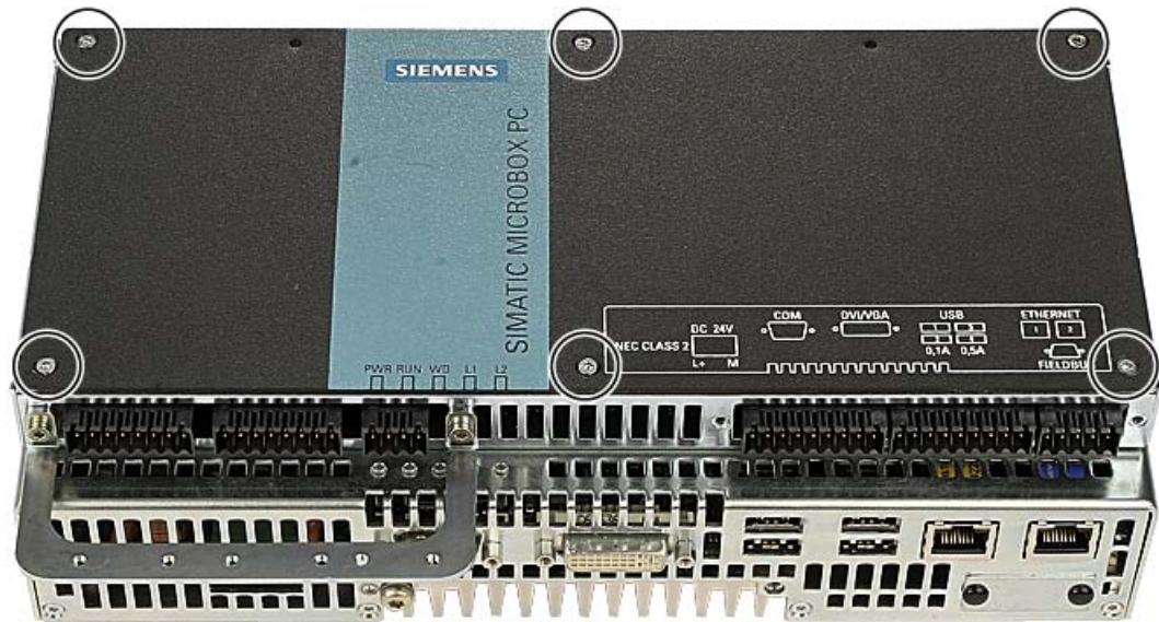
10. Stick the enclosed adhesive label showing the pin assignment of the I/O modules on the plug connections to the cover of the Microbox PC.
