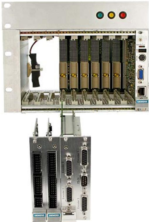
*6.2 Installation example: Basic module and two I/O modules*
