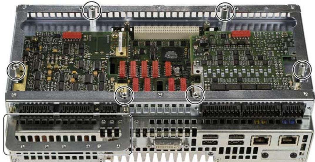
6. Tighten the shield clamp as shown in the diagram above. The shield clamp must be on the same side as the analog I/O module 0.
