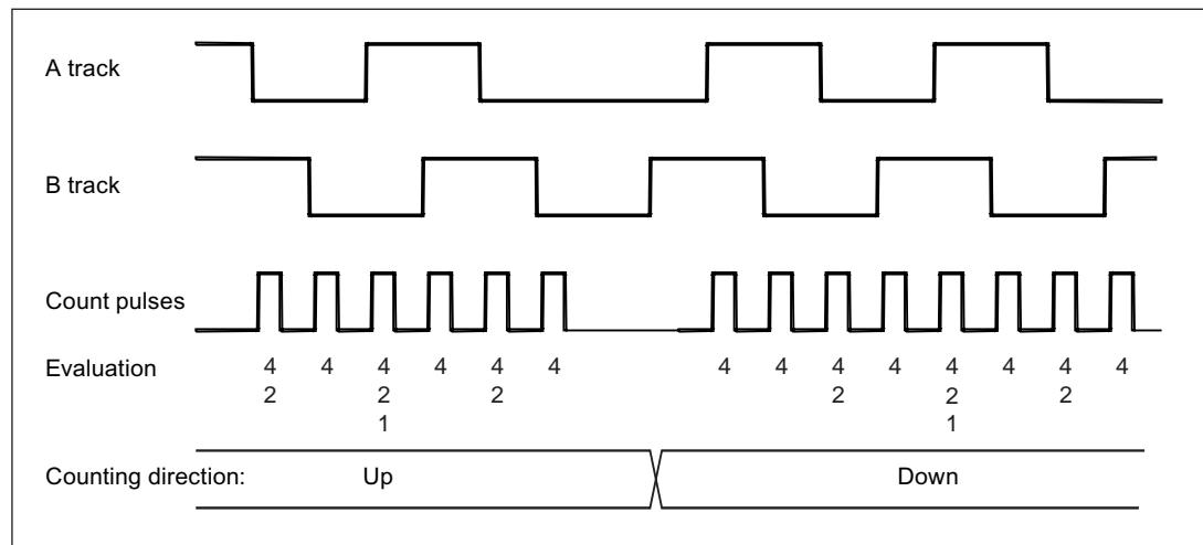
Figure 7-2 Shaft encoder edge evaluation with hysteresis function
