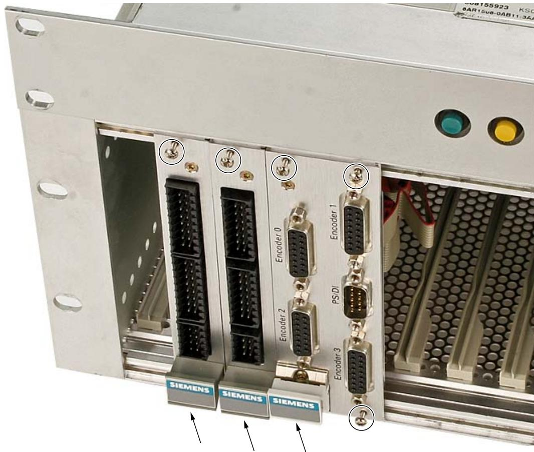
– Attach the shield of the analog signals to the frame of the mounting cabinet.
