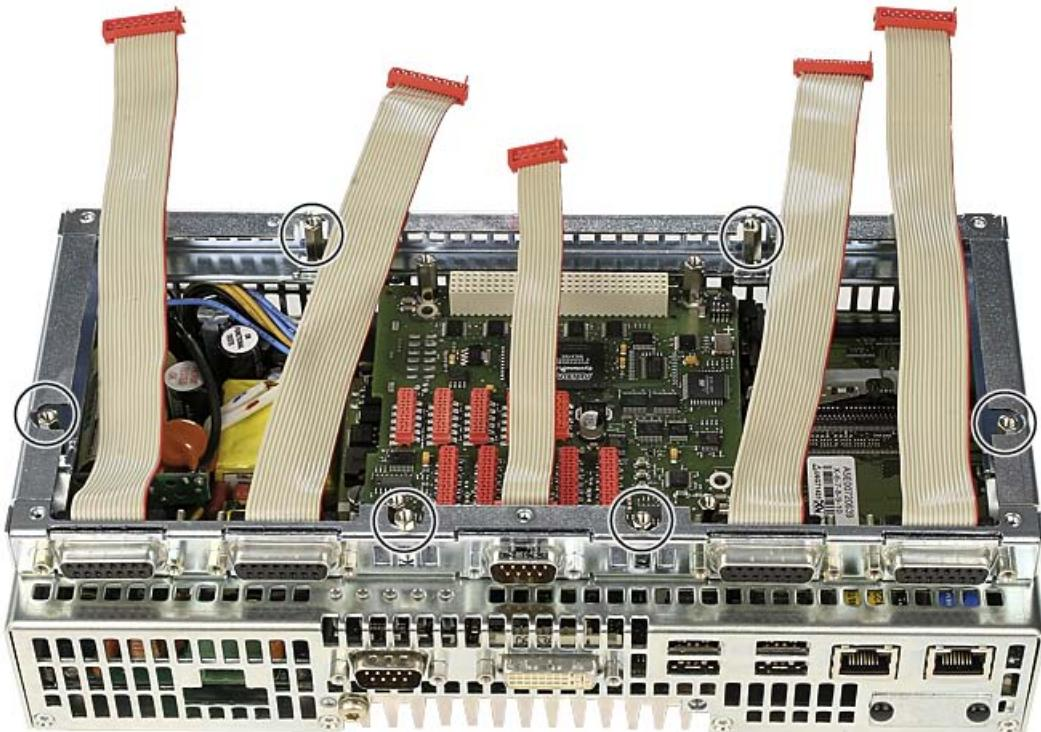
*5.3 Installation example: Basic module, encoder rack and four I/O modules*
