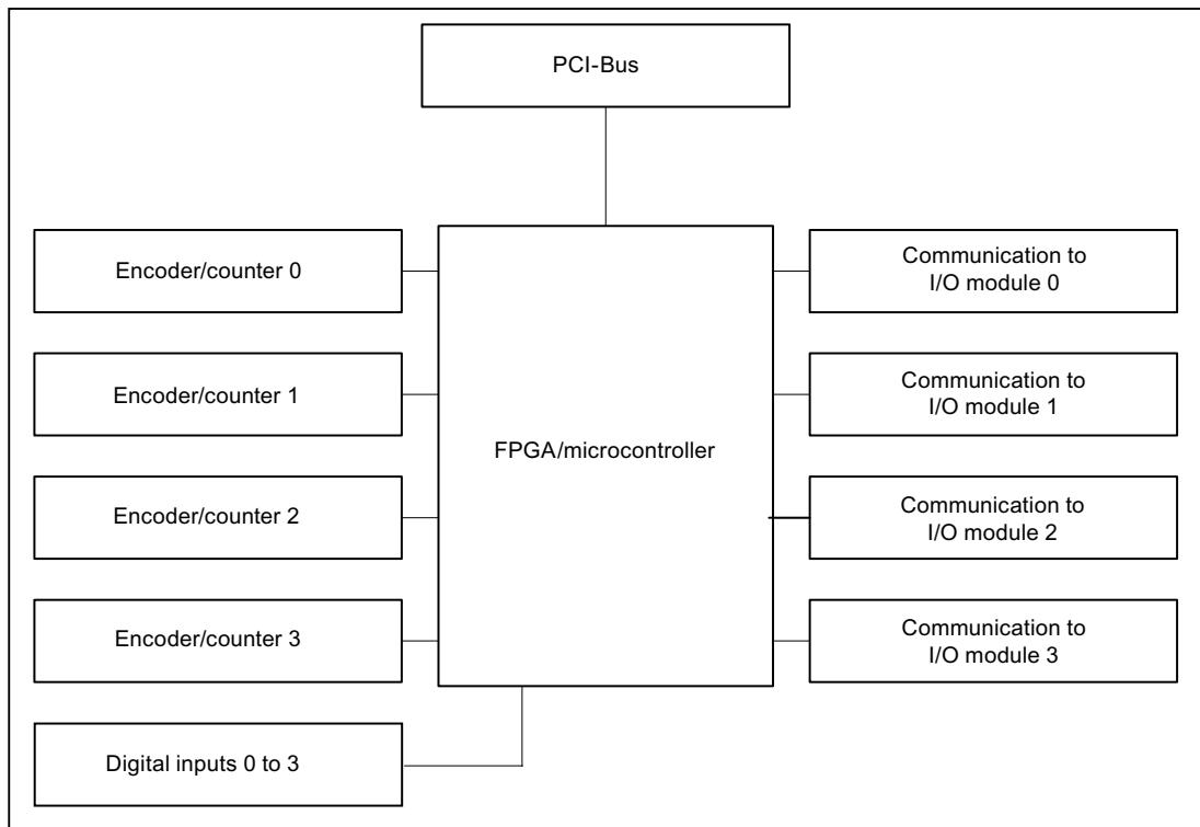
Figure 3-2 Function blocks of the basic module
