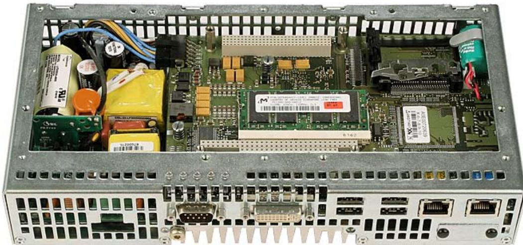
3. To set the slot, set the switch on the basic module to slot 0 (lowest slot). The procedure is described in "Preparatory work".
