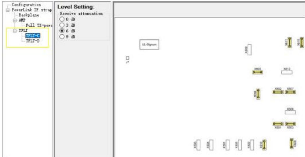
[isc_adjust_tflt_jumper_settings, 1, --] Figure 4-9 TFLT jumper settings
