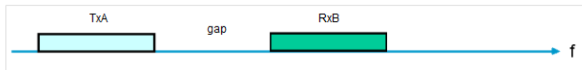
Figure 5-2 Example of an non-adjacent frequency bands location
