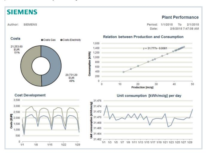
With the help of the regression analysis, a linear relationship between production and consumption is established. The calculation of the plant characteristic curve can be used both for forecasting and for baseline management.
