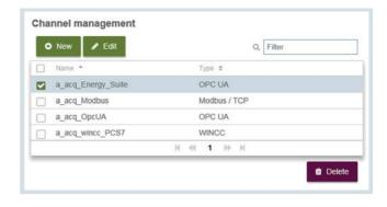
Depending on the type, a connection to a WinCC server, an OPC server or a Modbus device is required when creating a data channel. If you have created multiple data channels, you can display the data points from the specific data channels.
