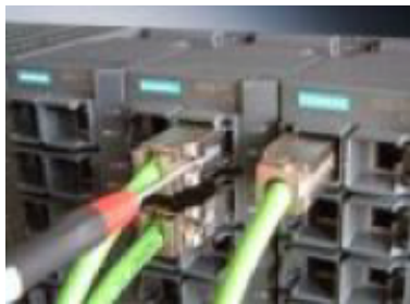
Figure 4-7 Releasing the RJ-45 Plug with a screwdriver
