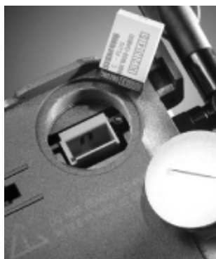
Figure 3-28 Removing the C-PLUG from the receptacle
