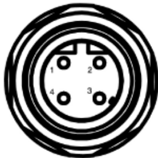
Figure 3-10 SCALANCE 208PRO Ethernet socket M12
