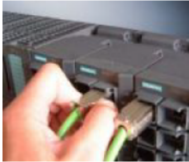
Figure 4-6 Releasing the RJ-45 Plug
