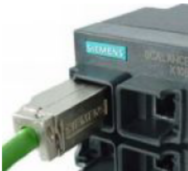
Figure 4-5 Inserting the IE FC RJ-45 Plug 180
