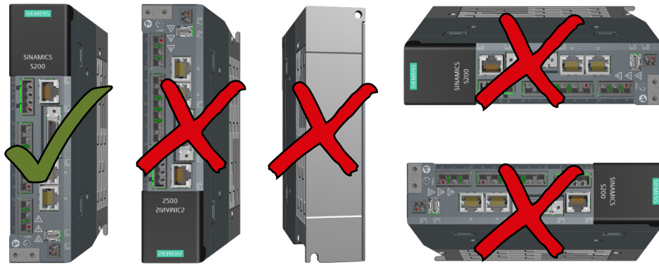
Figure 5-1 Converter mounting orientation
