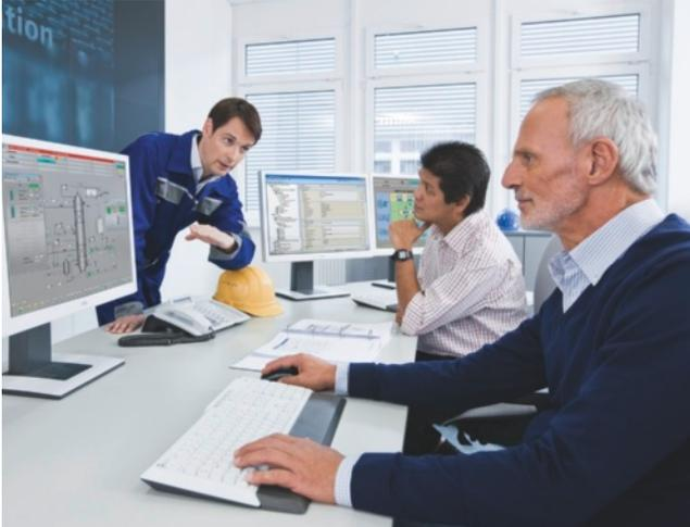
The SIMATIC PDM service and parameter assignment station can be used either locally or centrally. Both application scenarios can be combined in one system, e.g. an autonomous, stand-alone application in the field for the factory acceptance test (FAT) with centralized overall administration.
