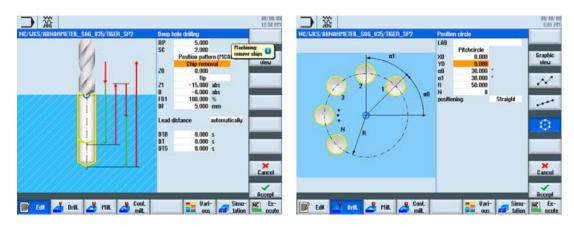
The SINUMERIK 828D offers you a unique range of CNC technology cycles for standard machining – including an engraving cycle. The assignment to the machining positions is performed very simply using a wide selection of ready position patterns, even with swiveled planes for milled workpieces.
