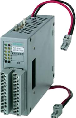
A Siemens SB61 interface module, similar in design to the SB60 but with a different internal configuration. It features a terminal block and a connector.                                      | <p>接口模块 SB61<br/>电气上隔离，完成信号转换48V-24V<br/>8数字输入，LED显示</p>  |
