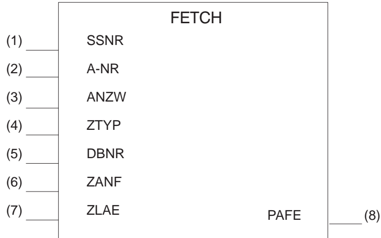
Figure 4-5 FETCH Function Block (FB 122)
