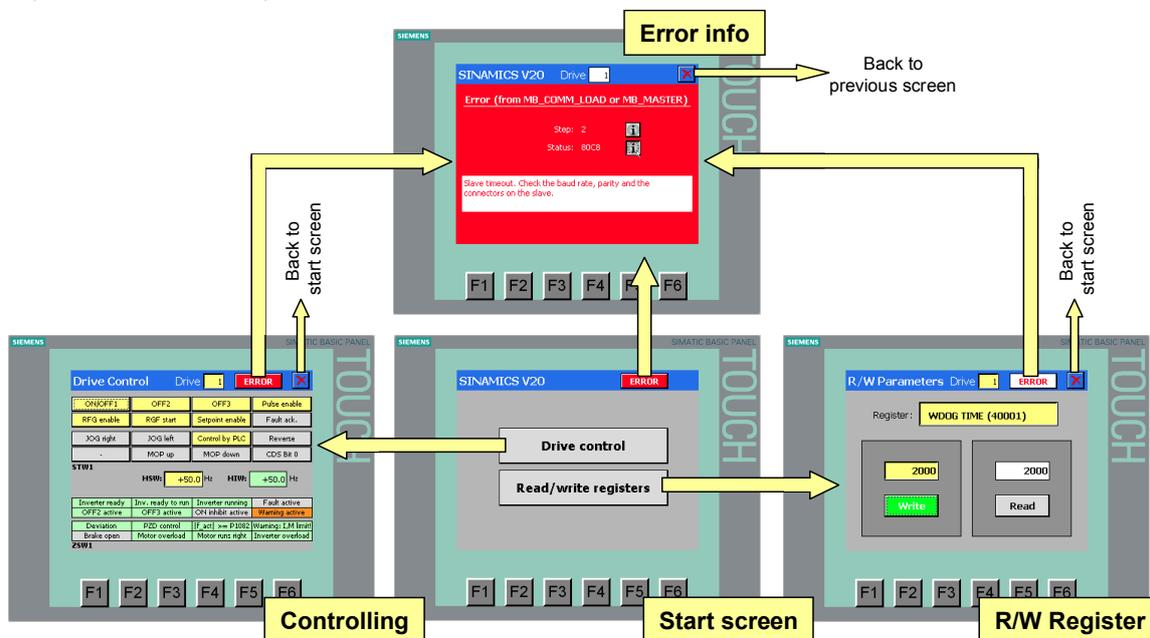
Select the desired function from the start screen. You get back to the start screen via the button in the respective function screen.
