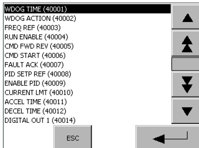
The list includes all registers that can be accessed at the SINAMICS V20 via the Modbus protocol. By selecting the register, the data format of the value to be read/written is also specified. If it is a “Read-only” parameter (rnnnn), the “Write button” is grayed out and any write attempt is stopped.
