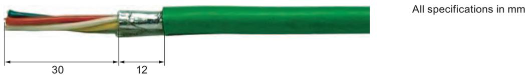
Figure 4-3 Stripping the PROFINET cable
