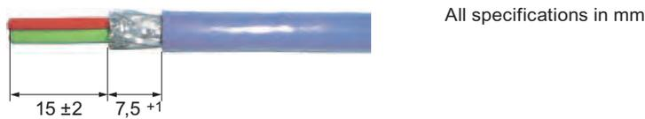
Figure 4-2 Stripping the insulation from the MPI/PROFIBUS-DP cable
