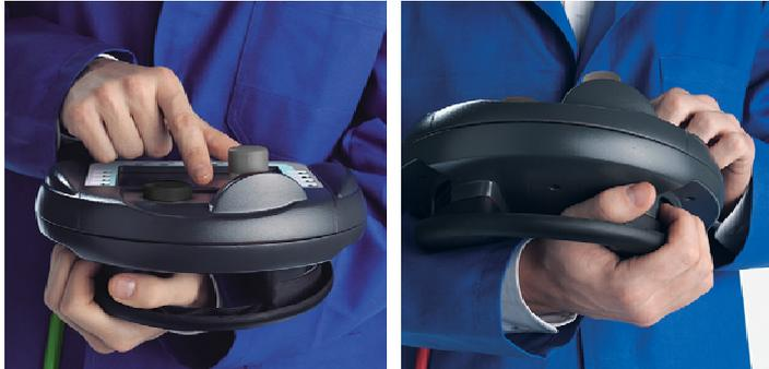
Figure 5-2 Example of forearm holding position for right or left-handed persons with Mobile Panel 177
