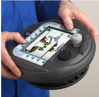
Figure 5-3 Example of two-hand holding on Mobile Panel 177
