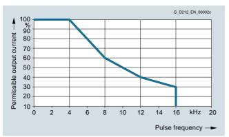
Output current as a function of pulse frequency (Single Motor Modules, 3 A to 132 A)
