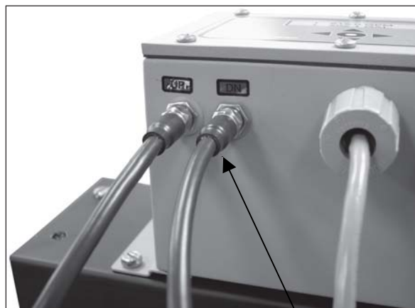
Figure 3 Connect Transducer Cables
