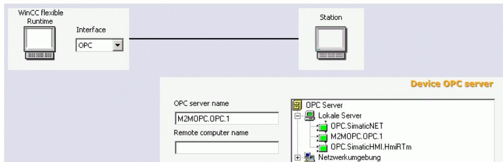
Figure 5-1: A server entry in WinCC flexible (example)
