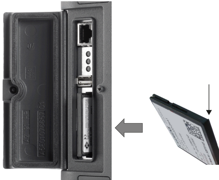
Figure 2-10 Direction to insert the user CompactFlash card
