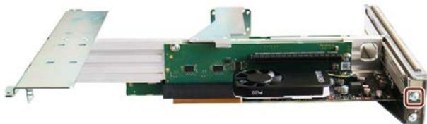
3. Remove the slot blanking panel.
