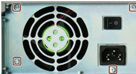
5. Pull the power supply upward and out of the housing.
