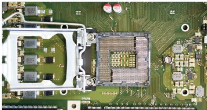
Note: The contact springs of the socket are highly sensitive to mechanical damage, e.g. caused by an incorrectly inserted CPU or foreign objects, and their entire surface may only touch the contact side of the processor flat.
