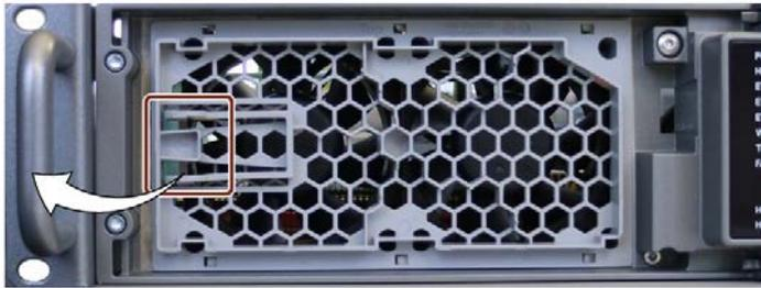
3. Set aside the fan support with the openings facing down right in front of the device. The fans are on top.
