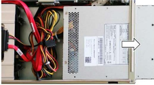
4. Remove the cable ties securing the power cables in the enclosure.
