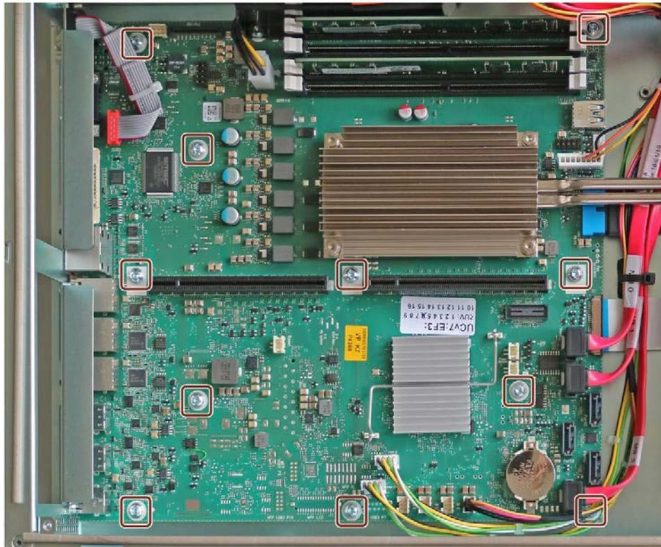
5. Remove the motherboard, install a new one and fasten it.
