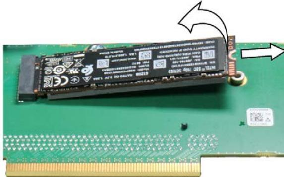
4. Place the thermal pad under the M.2 NVMe SSD and insert the M.2 NVMe SSD slightly inclined from above into the provided direct connector socket.
