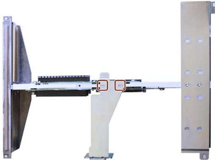
2. Remove the marked screws with which the piggyback is fixed to the center rail.
