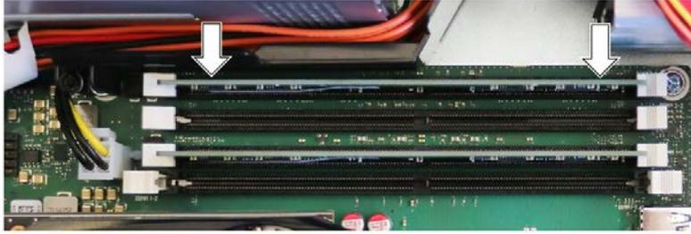
5. Press evenly on both sides of the memory module in order to prevent tilting until both interlocks audibly engage.
