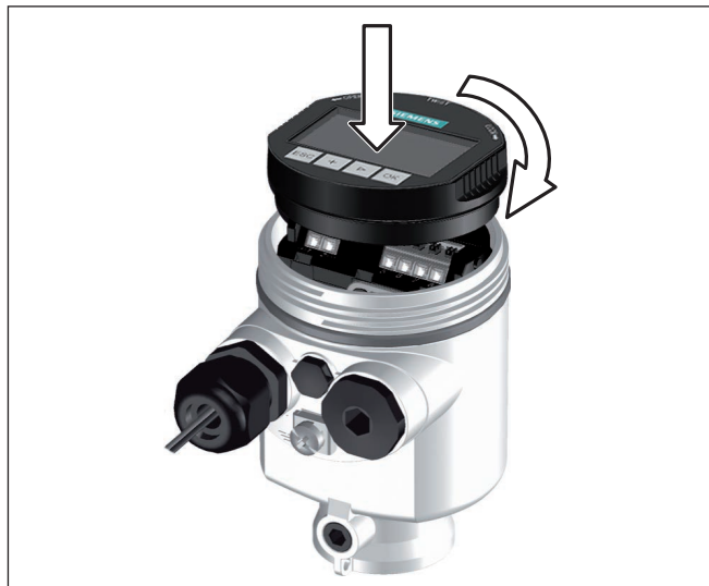
Fig. 23: Installing the display and adjustment module in the electronics compartment of the single chamber housing
