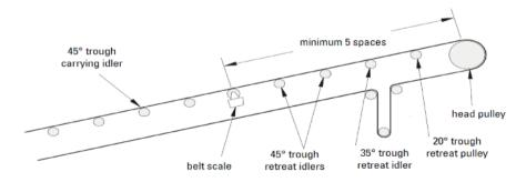
D. The vertical displacement of the head pulley relative to the adjacent retreat idler is normally in excess of what is acceptable for belt scale installations.
