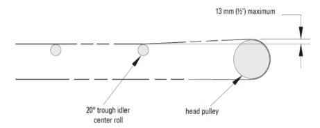
When locating a scale close to the head pulley, maintain a maximum of 13 mm (1/2") vertical displacement between the top of the head pulley and the top of the center roll of the adjacent idler by making the following adjustments:
