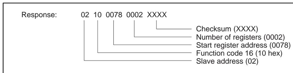
Figure 2-31 Write Multiple Registers Example — Response
