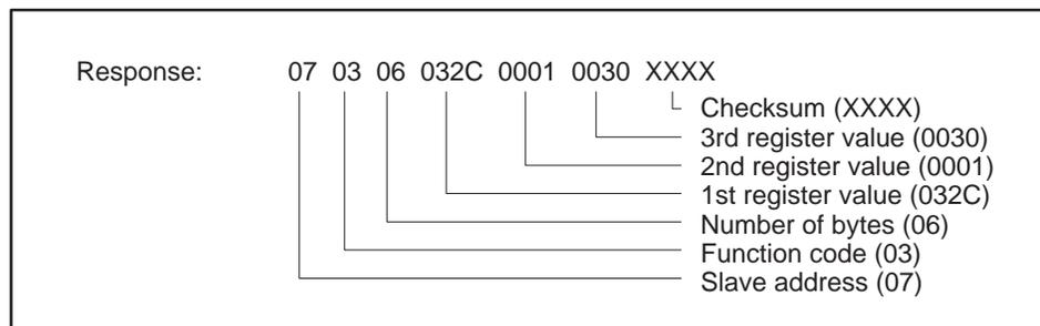
Figure 2-11 Read Output Register Example — Response
