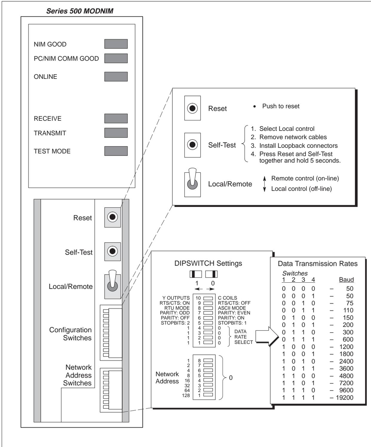
Figure 1-6 Series 500 MODNIM Switches and LEDs
