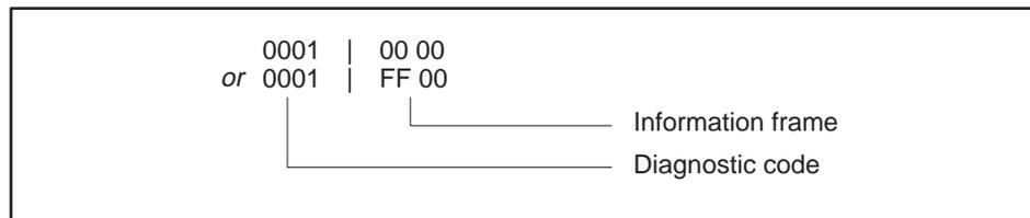
When Function Code 08 uses diagnostic code 0001, the information frame can contain 0000 or FF00.
