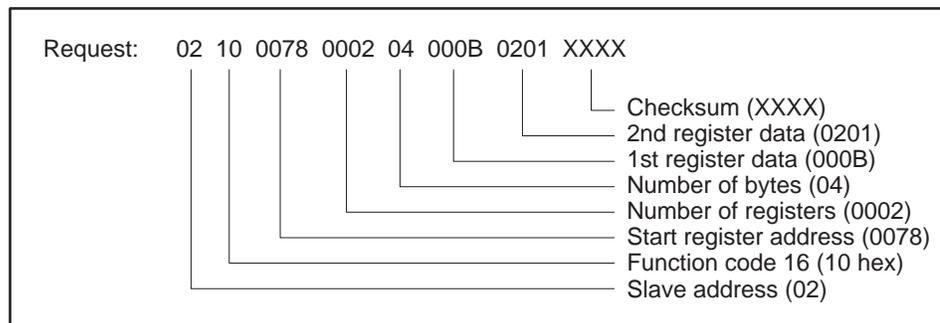
Figure 2-30 Write Multiple Registers Example — Request
