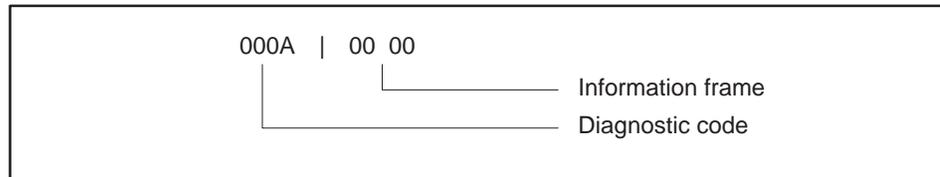
When Function Code 08 uses diagnostic code 000A and any value in the information field (00 00 shown), all diagnostic registers and counters within the MODNIM will be cleared. This also happens when the power is cycled or the RESET button is pressed.
