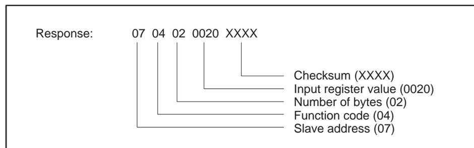
Figure 2-13 Read Input Register Example — Response
