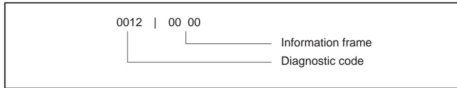
When Function Code 08 uses diagnostic code 0012 and any value in the information field (00 00 shown), the information field will return the number of character overruns detected by the MODNIM since the last RESET or power-up. This indicates the number of times that characters have arrived faster than the UART can store them without loss. The counter will increment to a value of FFFF (65535) and will then return to zero (0).
