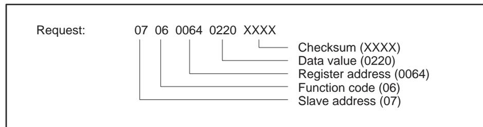
Figure 2-16 Write a Single Register Example — Request
