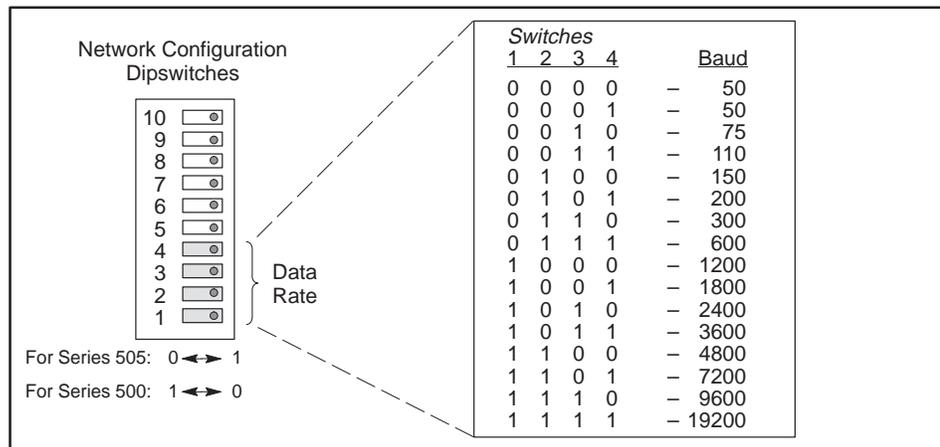
Figure 1-4 Dipswitch Settings for Network Data Transmission Rates
