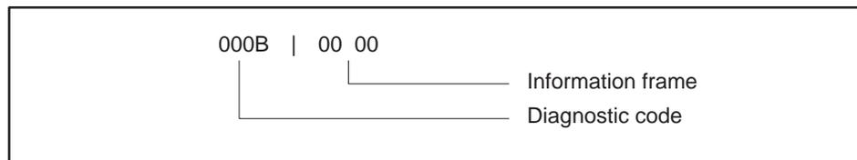
When Function Code 08 uses diagnostic code 000B and any value in the information field (00 00 shown), the information field will return the number of processed messages received by the MODNIM since the last RESET or power-up. The counter will increment to a value of FFFF (65535) and will then return to zero (0).
