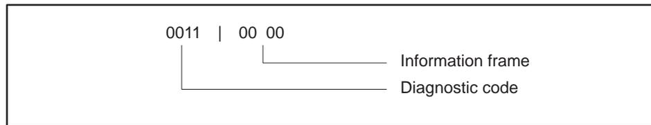
When Function Code 08 uses diagnostic code 0011 and any value in the information field (00 00 shown), the MODNIM will return 0000 in the information field.
