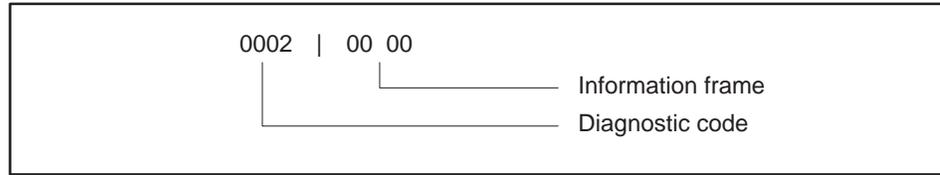
When Function Code 08 uses diagnostic code 0002, the information field may contain any value (00 00 shown). The MODNIM returns a 16-bit word containing diagnostic data about the attached device. The meaning of each bit is given in Table 2-5.
