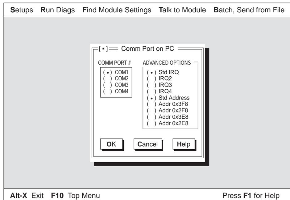
Figure D-1 First Configuration Screen after Start-Up
