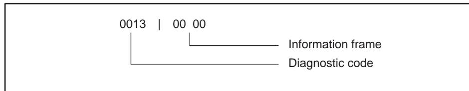
When Function Code 08 uses diagnostic code 0013 and any value in the information field (00 00 shown), the MODNIM will return 0000 in the information field.
