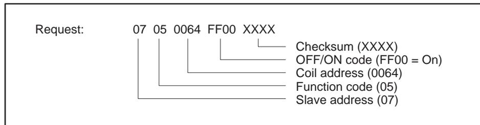
Figure 2-14 Write a Single Coil Example — Request
