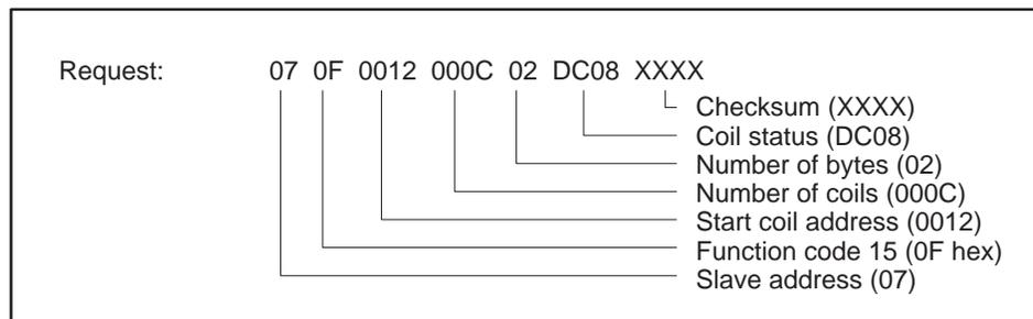
Figure 2-27 Write Multiple Coils Example — Request
