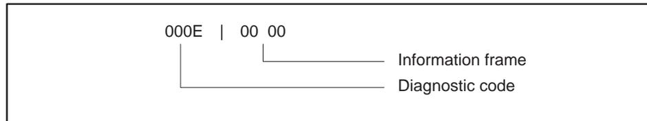
When Function Code 08 uses diagnostic code 000E and any value in the information field (00 00 shown), the information field will return the number of messages addressed to the MODNIM since the last RESET or power-up. The counter will increment to a value of FFFF (65535) and will then return to zero (0).
