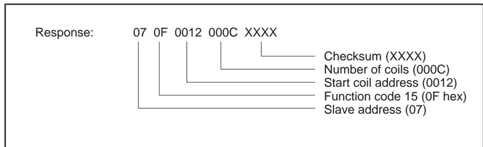
Figure 2-29 Write Multiple Coils Example — Response
