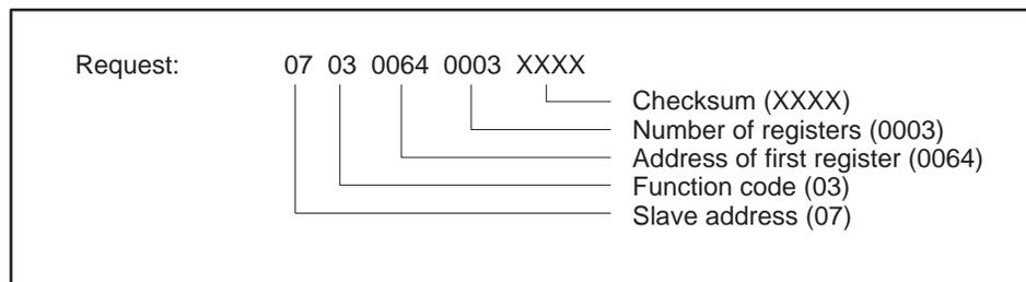
Figure 2-10 Read Output Register Example — Request
