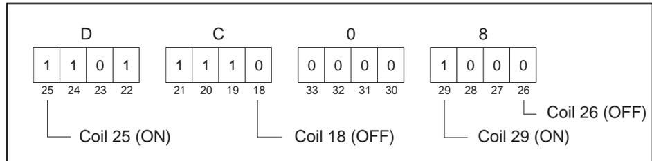
Figure 2-28 Coil Bit Pattern
