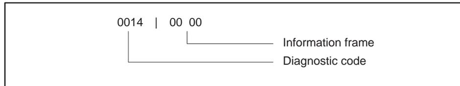
When Function Code 08 uses diagnostic code 0014 and any value in the information field (00 00 shown), the MODNIM will clear the character overrun counter.
