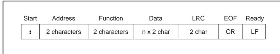
Figure 2-1 ASCII Transmission Frame
