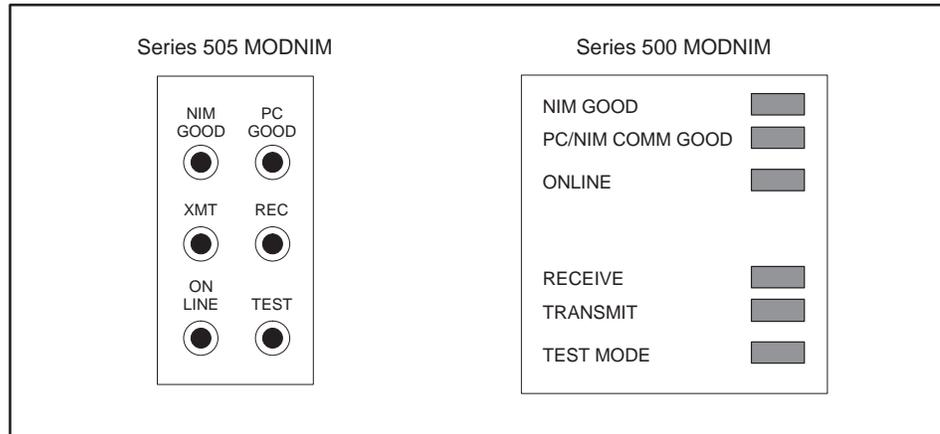
Figure 1-11 Series 505 and 500 MODNIM Indicator Lights
