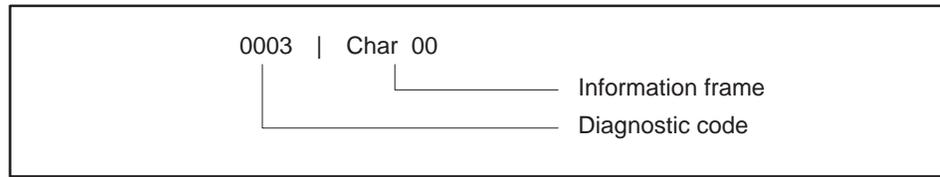
When Function Code 08 uses diagnostic code 0003, the ASCII character given in the information field is then used as the delimiter of an ASCII mode message replacing the standard LF (line feed) character.
