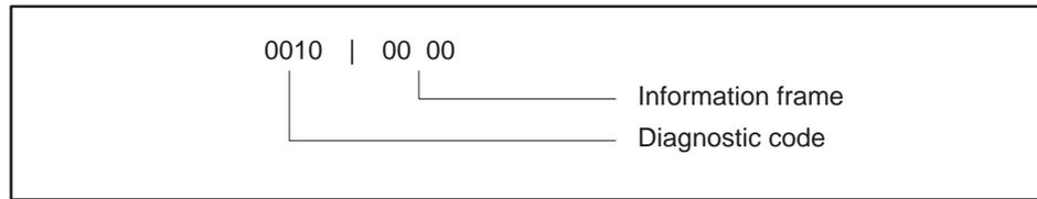
When Function Code 08 uses diagnostic code 0010 and any value in the information field (00 00 shown), the MODNIM will return 0000 in the information field.
