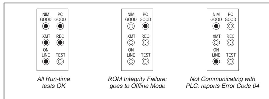
Figure 1-13 LED Status during Normal Run-Time Operation
