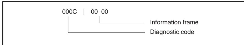
When Function Code 08 uses diagnostic code 000C and any value in the information field (00 00 shown), the information field will return the number of checksum errors detected by the MODNIM since the last RESET or power-up. The counter will increment to a value of FFFF (65535) and will then return to zero (0).
