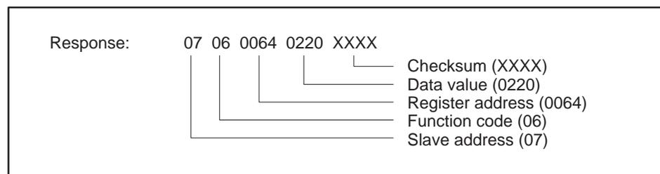
Figure 2-17 Write a Single Register Example — Response
