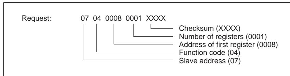
Figure 2-12 Read Input Register Example — Request
