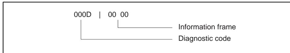
When Function Code 08 uses diagnostic code 000D and any value in the information field (00 00 shown), the information field will return the number of exceptions detected by the MODNIM since the last RESET or power-up. The counter will increment to a value of FFFF (65535) and will then return to zero (0).
