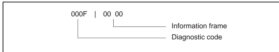
When Function Code 08 uses diagnostic code 000F and any value in the information field (00 00 shown), the MODNIM will return 0000 in the information field.
