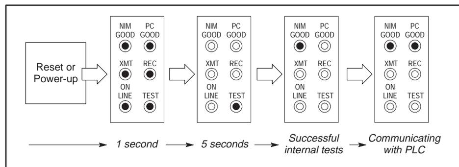
Figure 1-12 LED Status during Power-Up Self Test
