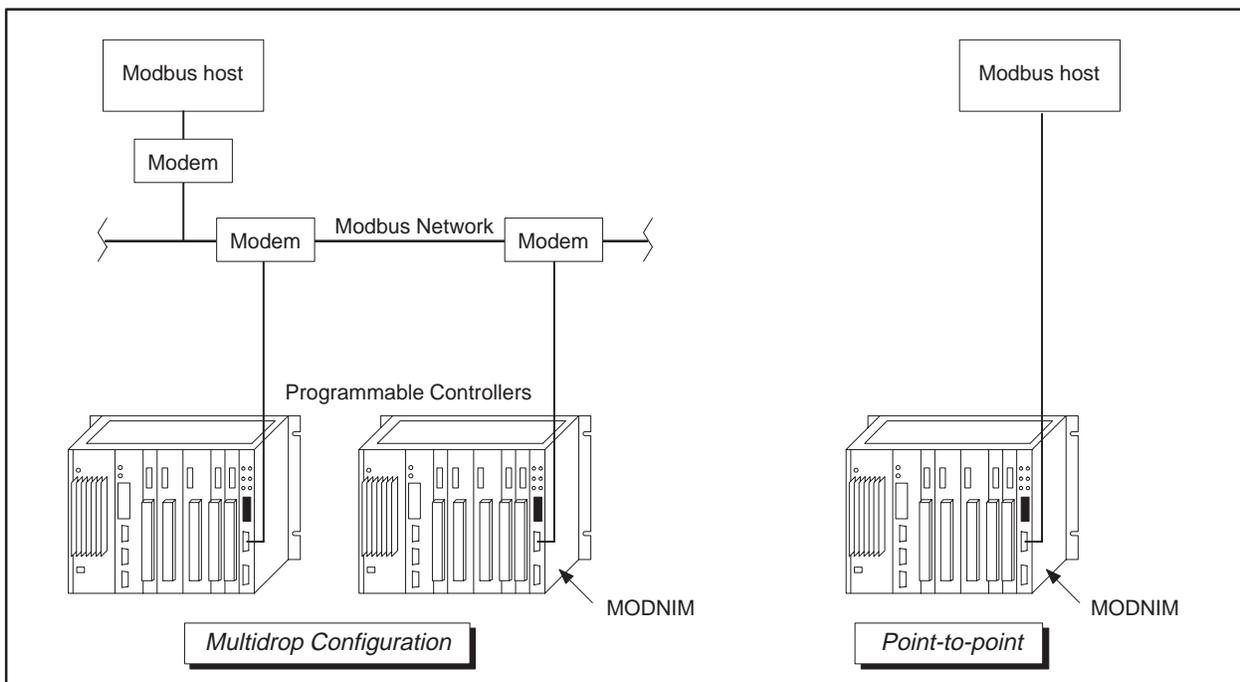
Figure 1-1 Multidrop and Point-to-point Configurations
