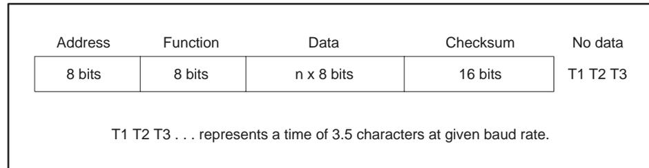
Figure 2-2 RTU Transmission Frame
