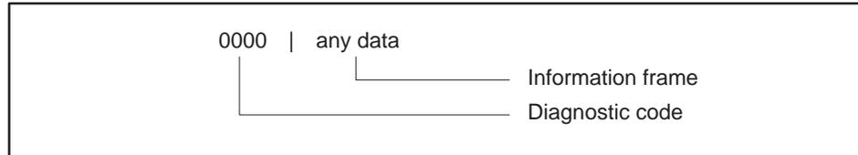
When Function Code 08 uses diagnostic code 0000, any data passed in the information field is returned to the host computer by the addressed secondary node without change.
