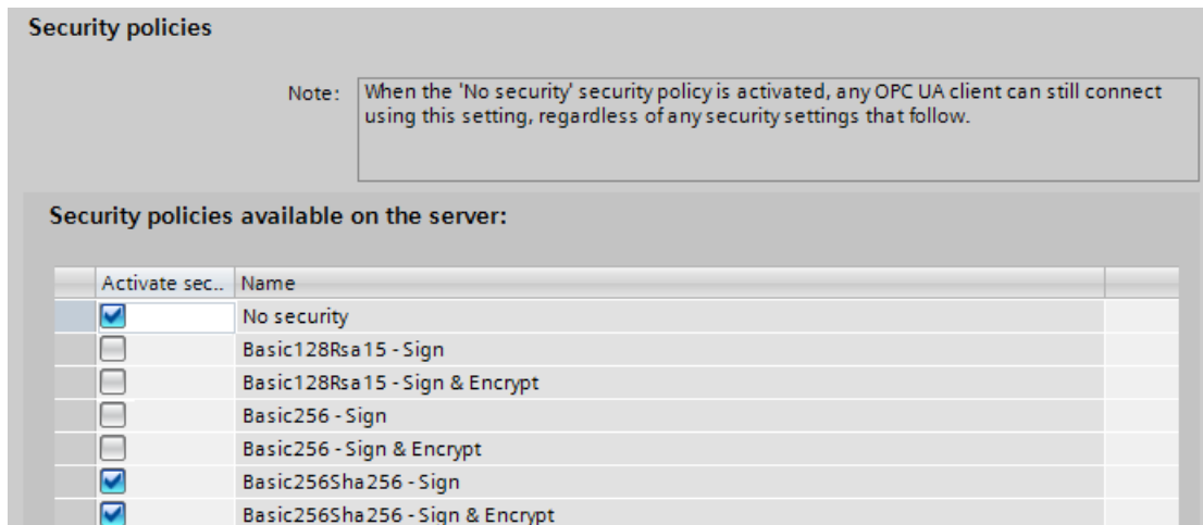
Figure 11-28 Configuring security settings of the server
