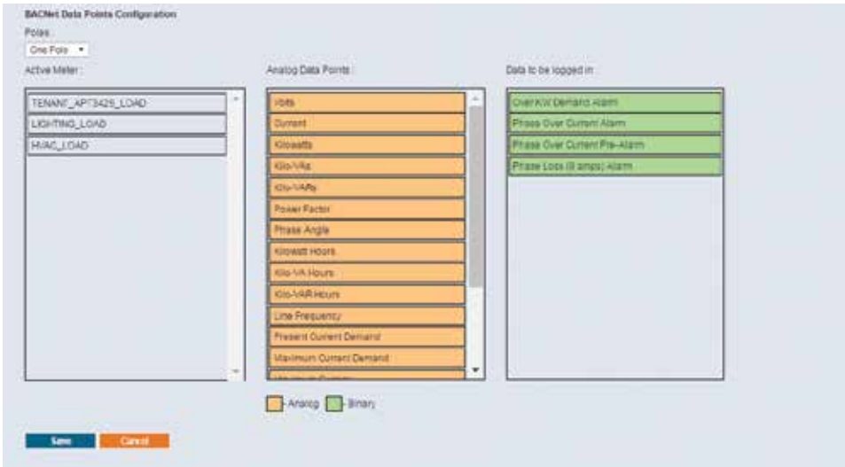
BACnet Data Logs Page (BACnet IP)
