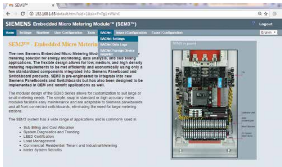
Navigating to BACnet Settings Page (BACnet IP)
