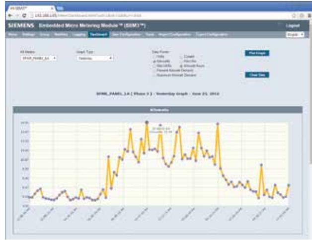
The SEM3 dashboard can also take one metered point and look at a variety of values for that one point. This information can be used to smooth usage or to identify potential issues early to turn into preventive actions.
