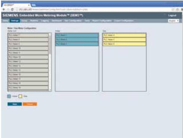
Water and Gas inputs – Using the S7 1200 PLC in conjunction with the SEM3 system up to 22 water and 22 gas pulse input can be incorporated into a utility management system. This give the building manager one place to see all the energy inputs in one place. The S7 1200 PLC can also be on its own separate UPS ( purchase separately)to continue counting pulses when the electricity is down.
