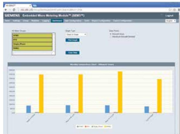
The SEM3 dashboard allows the data to be seen in multiple formats to make analytics easier to visualize. Whether you are looking at load trends of total consumption for multiple points the dashboards are a quick and easy tool to help visualize your electrical system.
