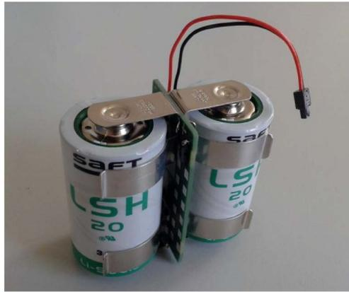
Figure C-4 Battery holder with batteries inserted
