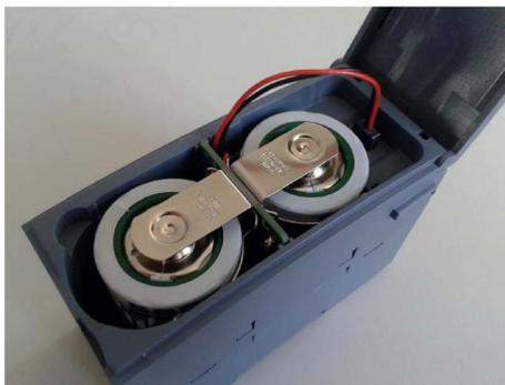
Figure 3-12 Battery module (not mounted) with inserted battery holder, cable connected.
