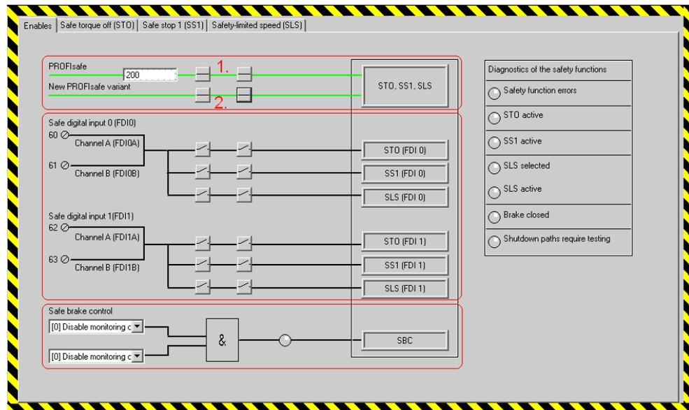
In this screen parameterize which source (**PROFIsafe** or the **Safe digital inputs**) is used to activate the safety functions of SINAMICS G120.
