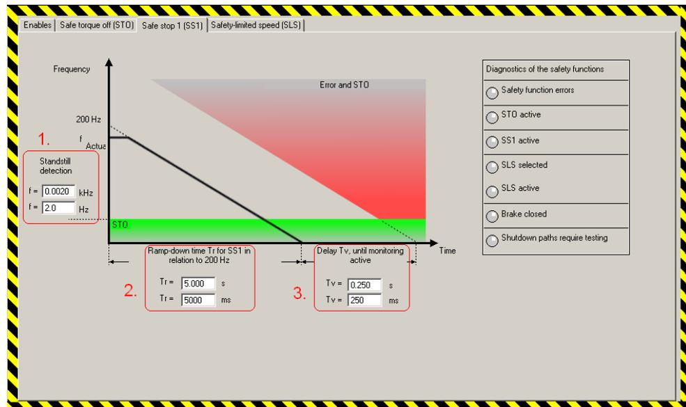
The parameters relevant for "Safe Stop 1" (SS1) are set in this screen form.
