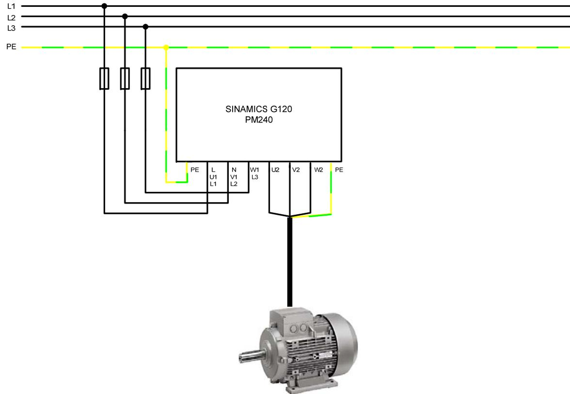
For more detailed information regarding the installation please refer to the **SINAMICS G120 Hardware Installation Manual Power Module PM240**. Download from: <http://support.automation.siemens.com/WW/view/en/22339653/133300>
