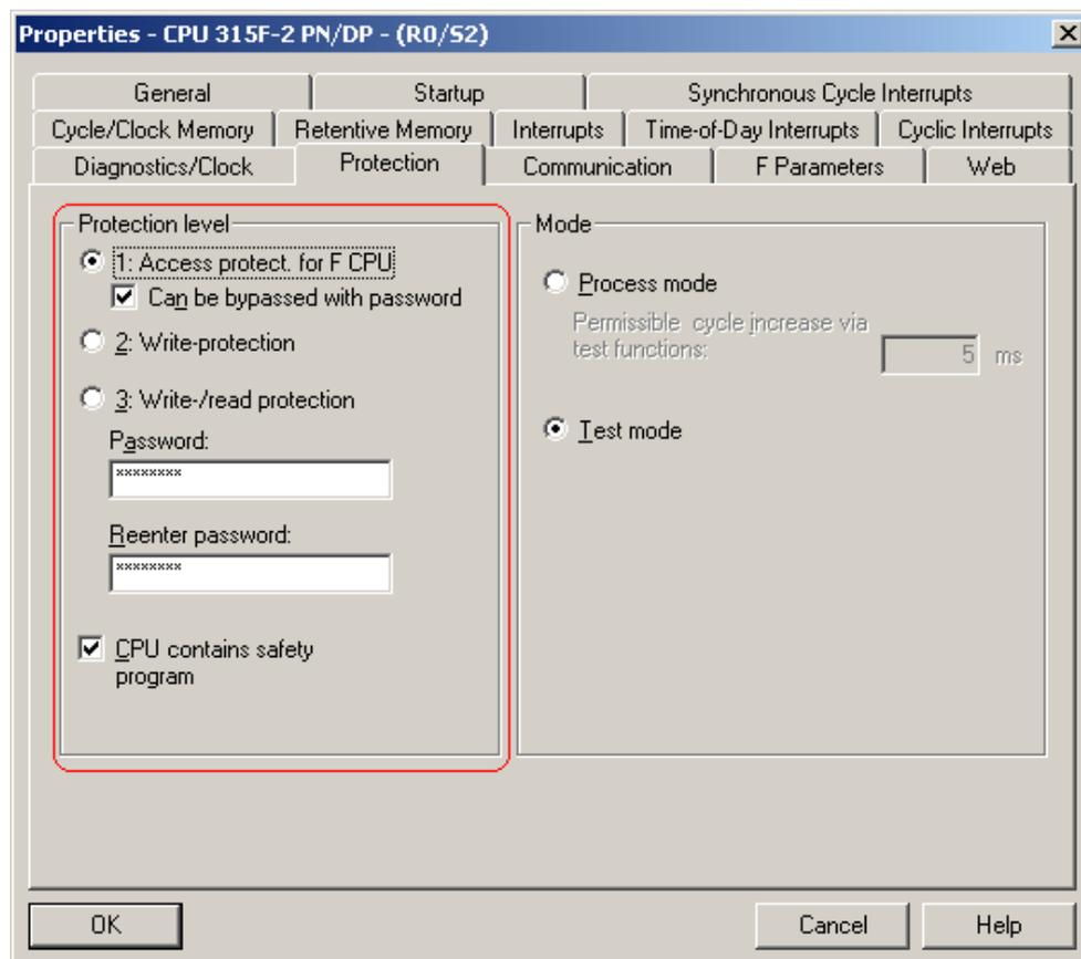
Under the **Protection** tab, the safety functions of the CPU are enabled by selecting the following functions:
