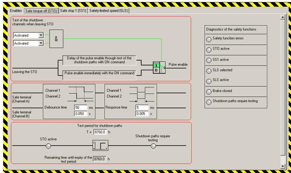
The shutdown paths of a safety-relevant plant or system must be subject to a forced checking procedure at regular intervals. This is in order to identify "dormant" errors. SINAMICS G120 automatically carries out a forced checking procedure of the shutdown paths in the drive unit. This procedure is known as the forced checking procedure.
