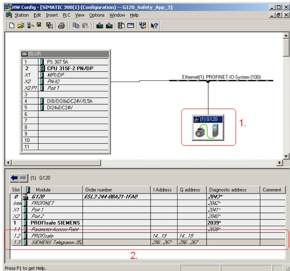
The PROFIBUS telegram (2.) between the CPU and the SINAMICS G120 comprises two components. One is the **Standard Telegram**, in this particular example, **Standard Telegram 352** for the communications of the SINAMICS G120 (control signals, status signals, frequency setpoint, frequency actual value etc.) and the other is the **PROFIsafe** for PROFIsafe communications.
