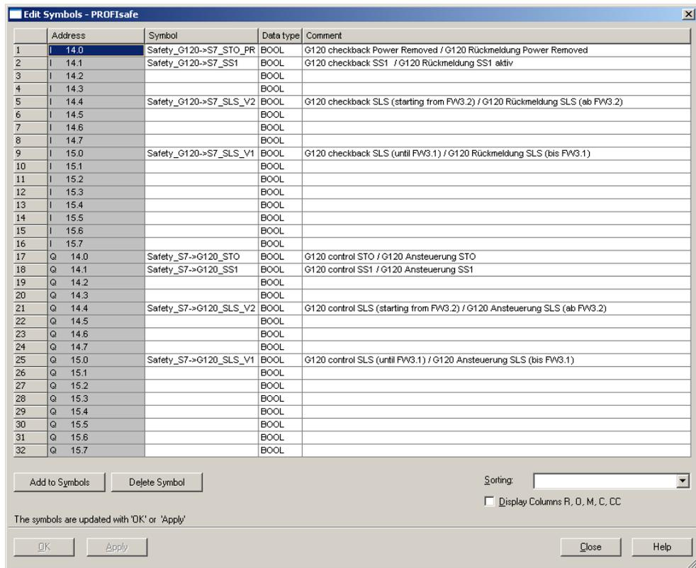
Only the inputs and outputs listed in this example are relevant for communications.
