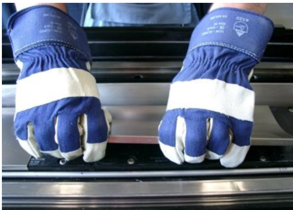
Figure 4-10 Dismounting a segment of the segmented secondary section cover
