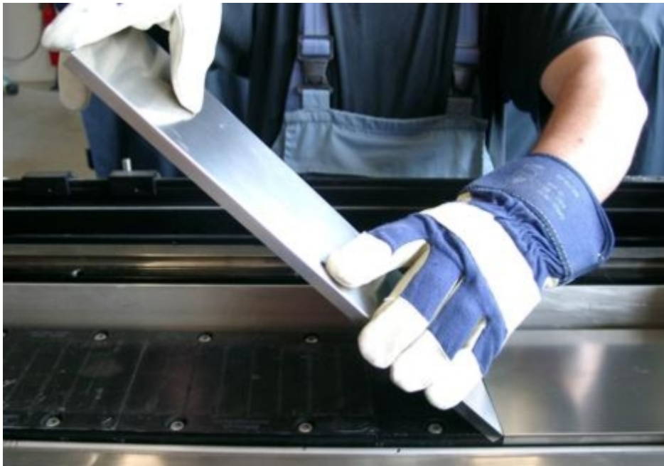
Figure 4-9 Mounting of a further segment of the segmented secondary section cover
