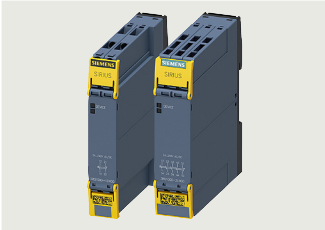
Picture on left: 3RQ1000-1EW00 coupling relay, 1 NO contact + 1 NC contact, screw terminal Picture on right: 3RQ1000-2LW00 coupling relay, 4 NO contacts + 1 NC contact, spring-loaded terminal (push-in)
