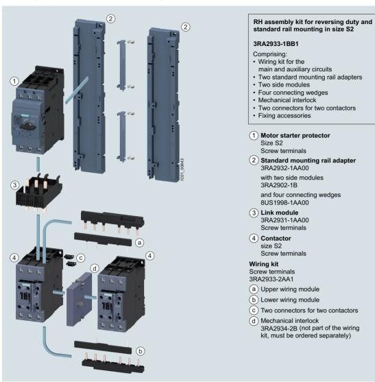
3RA22 load feeder for reversing duty and standard rail mounting in size S2 (the version with screw terminals is shown in the picture)
