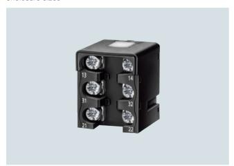
The three-pole contact block with snap-action or slow-action contacts is regularly available for all enclosure forms. The same installation space is required as for a two-pole block. The version with 1 NO + 2 NC offers, for example, more safety through redundant shutdowns (2 NC contacts) with simultaneous signaling (NO contact). The three-pole blocks are also available with make-before-break and with 2 NO + 1 NC.
