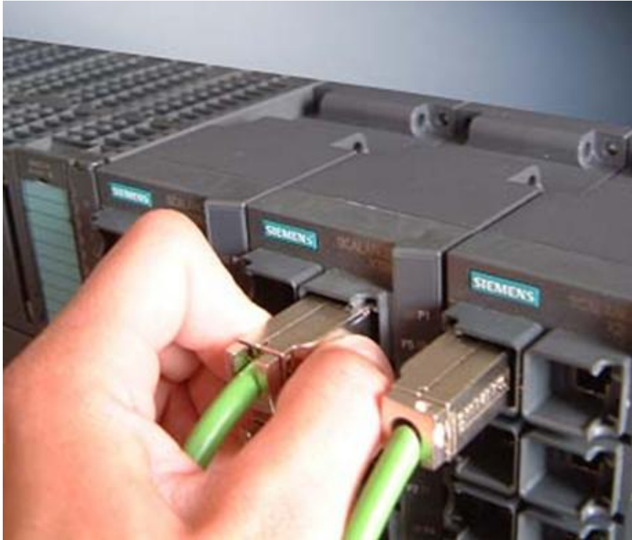
Figure 4-6 Unlatching the RJ-45 plug
