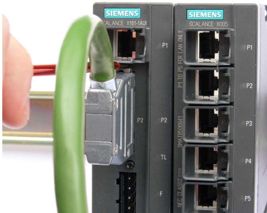
Figure 4-8 Locking or unlocking the SUB-D connector
