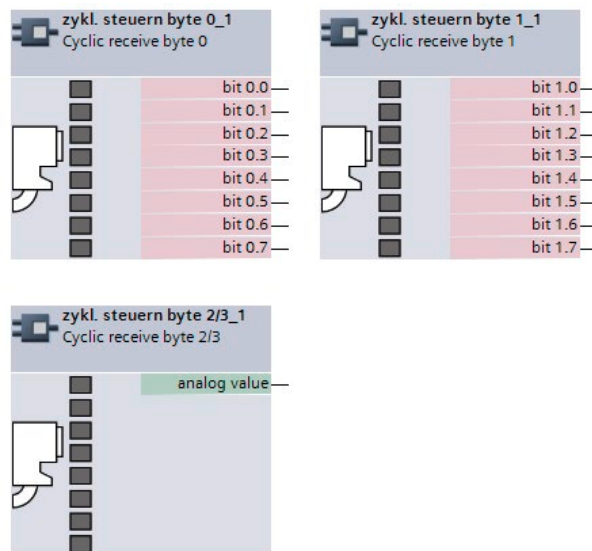
Figure 2-11 Cyclic data to SIMOCODE pro, basic type 1, 4 bytes
