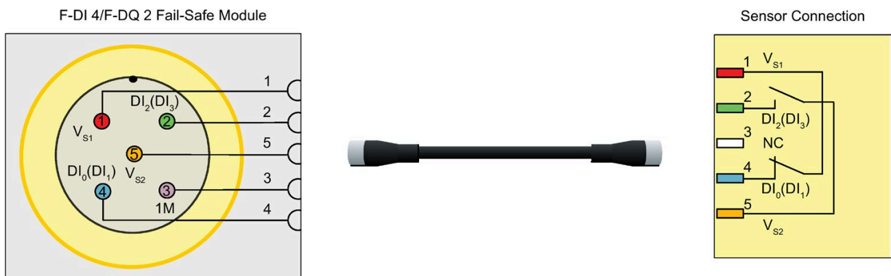
Figure 5-10 F-DI application mode 7: Internal sensor supply (1oo2 evaluation of two-channel sensor with nonequivalent outputs shown)
