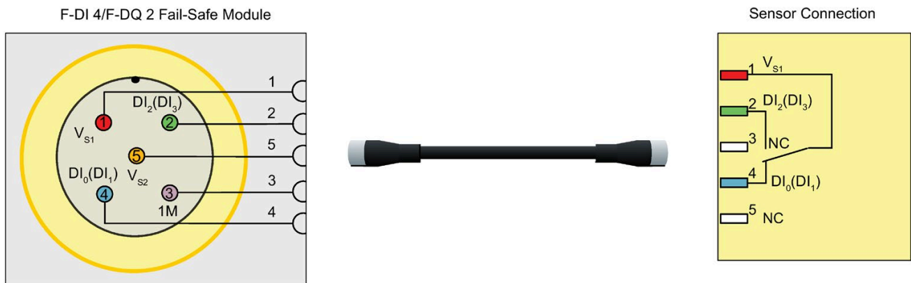
Figure 5-7 F-DI application mode 5: Internal sensor supply (1oo2 evaluation of two-channel sensor with nonequivalent outputs shown)
