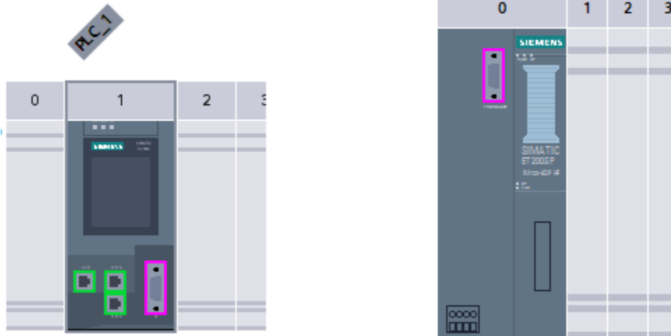
Figure 2-4 PROFIBUS DP interfaces
