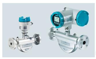
The complete flowmeter system SITRANS FC consist of a new FCS400 sensor in sizes DN 15 to DN50 mm and a FCT030 multichannel/multifunctional in compact or remote versions, or a single Modbus-channel FCT010 transmitter in compact version. The flowmeter is based on the latest developments within digital signal processing technology – engineered for high measuring performance:
