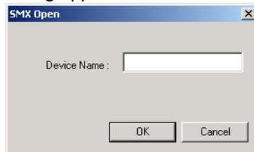
The Device Name field on the SMX Open dialog contains the controller name as specified in the Station Configuration Editor. The default device name is WinLC RTX.
