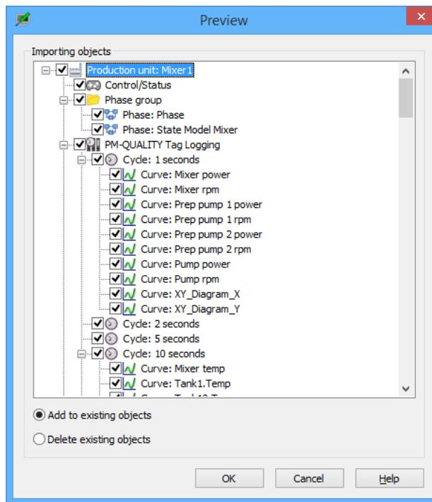
Figure 23: Example for importing a production unit
