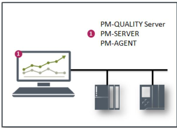
Figure 6: PM-QUALITY single-user system on a local base system
