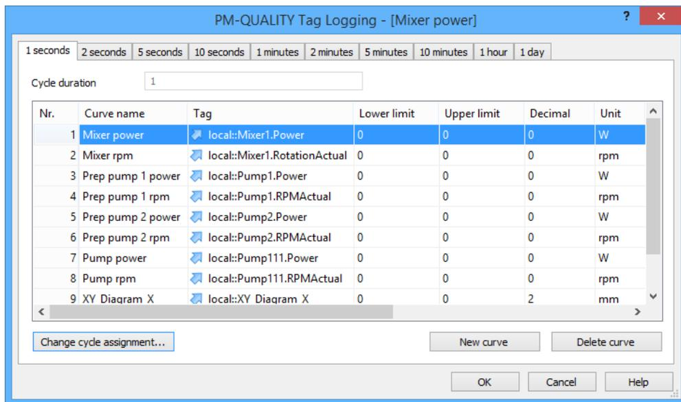
Figure 17: Configuration PM-QUALITY Tag Logging
