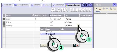
Alarms always belong to an alarm class. You define specific properties for each alarm class, for example, the color of acknowledgement states. A specific alarm class is always logged to a particular log file.
