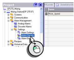
4. Configure the "Error" alarm class so that the alarms are logged to the "Mixer\_Speed" alarm log.
