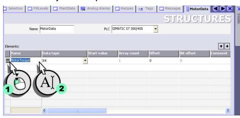
3. In the same way, create the entries for the motor temperature and the motor current:
