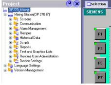
The larger display has enabled the engineering service to display the fill level indicator in closer detail. Open the "FillLevels" screen and see for yourself:
