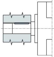
Align the offset at the coupling between electrical machines and the driven machines so that the maximum permissible vibration values according to ISO 10816-3 are not exceeded.
