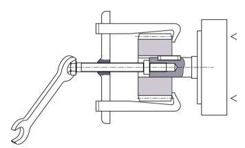
Withdrawing drive output elements
