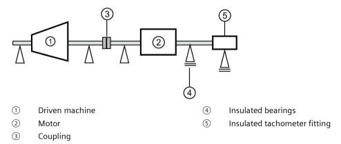
Figure 4-2 Schematic representation of a single drive
