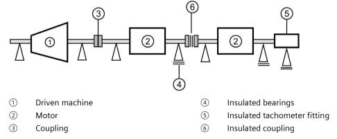
Figure 4-3 Schematic representation of a tandem drive
