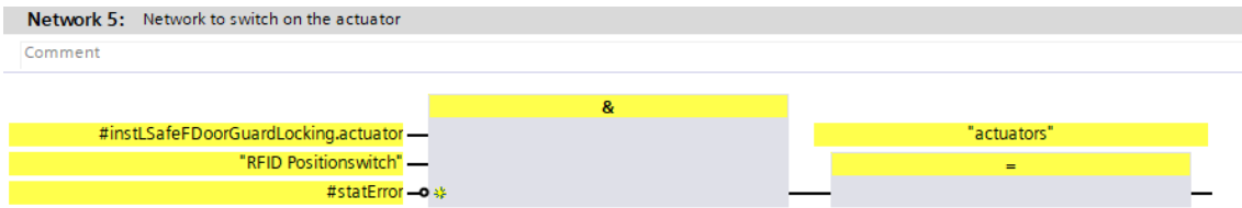
Figure 3-11 Checking the switch-on conditions for the actuator
