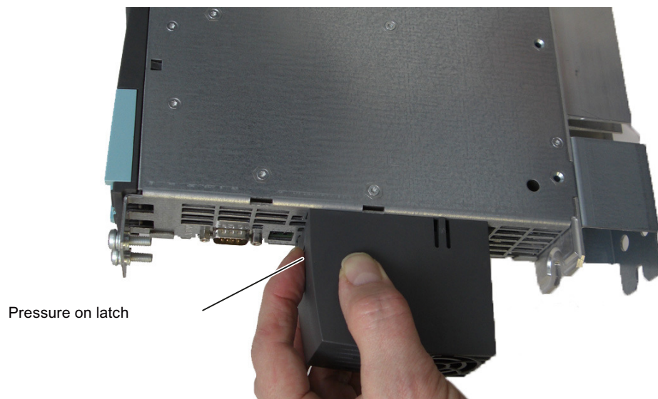
Figure 8-2 Unlatching the fan/battery housing
