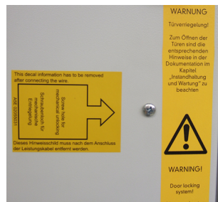
Figure 4-7 Example: Cover screw for manual door interlocking
