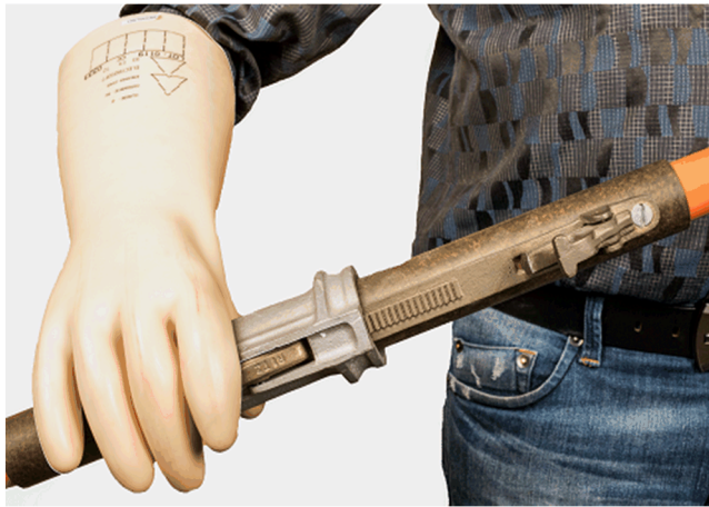
Figure 3-18 Locking the Jaw Hook of the Hot Stick with Shotgun
