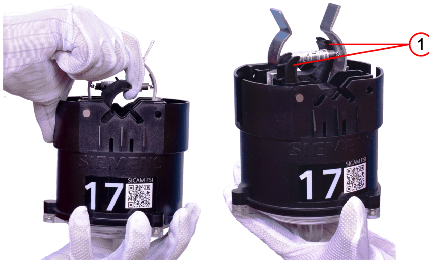
Figure 3-14 Opening the Hooks of the Device
