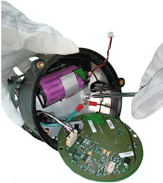
Figure 8-5 Fitting the Voltage Detection Plate in the Housing
