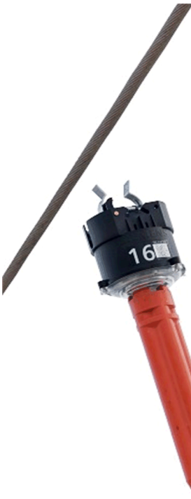
Figure 3-19 Mounting the Device on the MV Overhead Line
