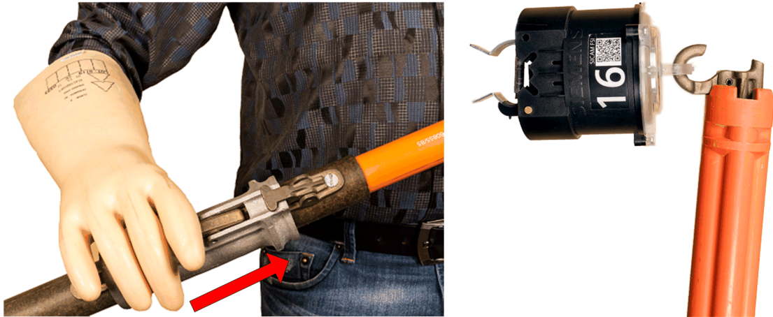
[dw_fsi_devopen-20160620_2_en_US] Figure 3-16 Opening the Jaw Hook of the Hot Stick with Shotgun
