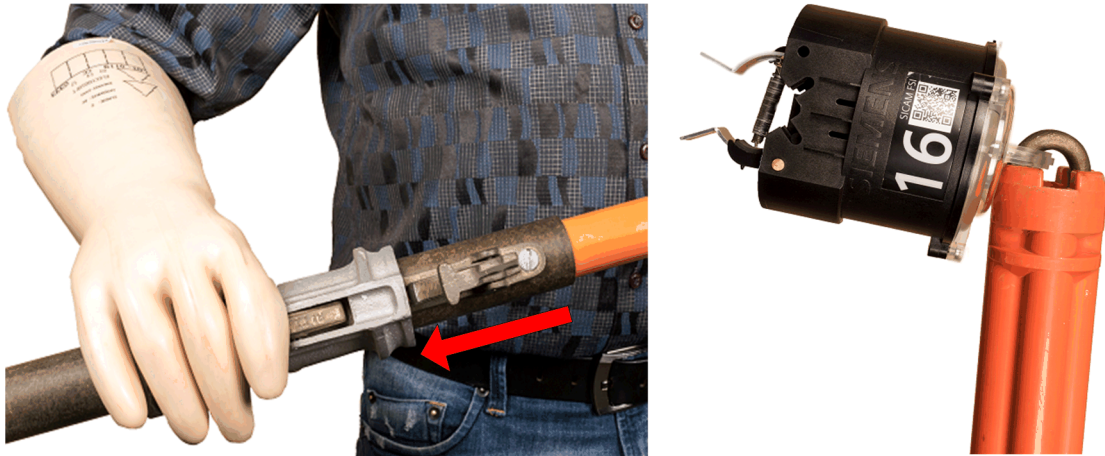
[dw_fsi_devdose-20160620_2_en_US] Figure 3-17 Closing the Jaw Hook of the Hot Stick with Shotgun
