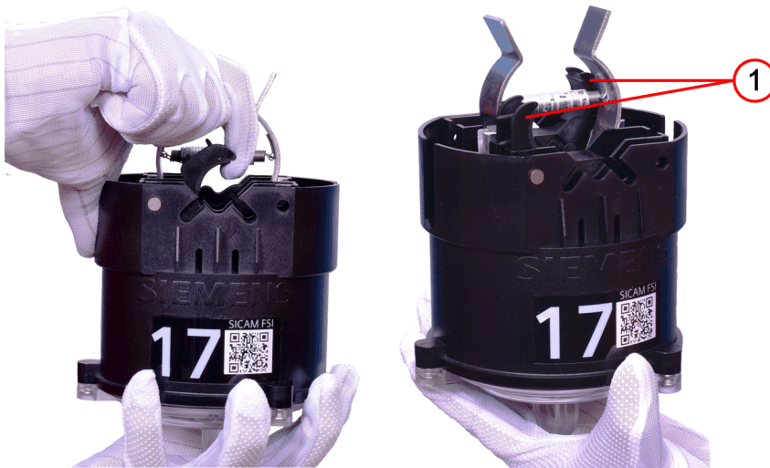
Figure 3-23 Opening the Hooks of the Device
